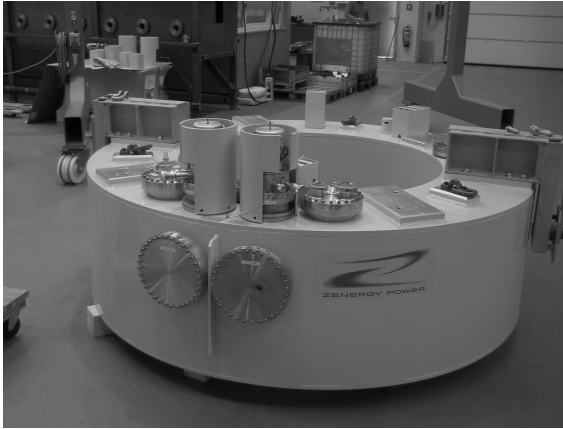
9.13 One of the two ASL/Zenergy superconducting magnets for the SFCL at CE electric. The coil uses a BSCCO-2223 from American Superconductor. It can produce a magnetic field over 2T and fully saturates the iron cores in the tank shown in the previous slide. This picture shows power leads for the coil and the flanges where two refrigerators will be installed.
