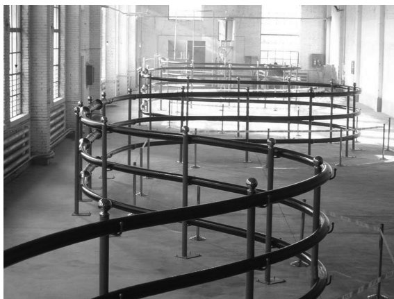
9.24 Test installation of the three phases of the Changtong warm dielectric HTS cable at the Changtong Cable plant in Baiyin, China. This cable is now installed at the 12.5 kV substation in Baiyin city, Gansu province. (Source: Courtesy Changtong Cable.)
