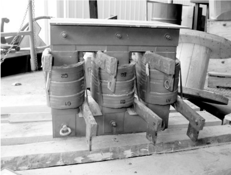
Figure 6.8 Photograph of a 0.047 mH three-phase line reactor.
