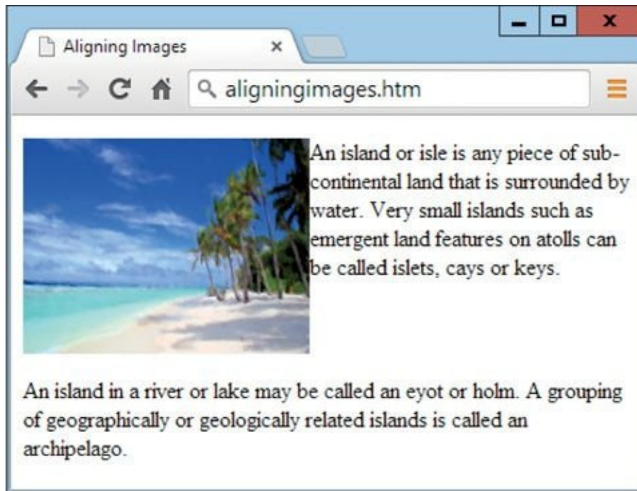
FIGURE 4-4 The left alignment is cleared before the start of the second paragraph.
