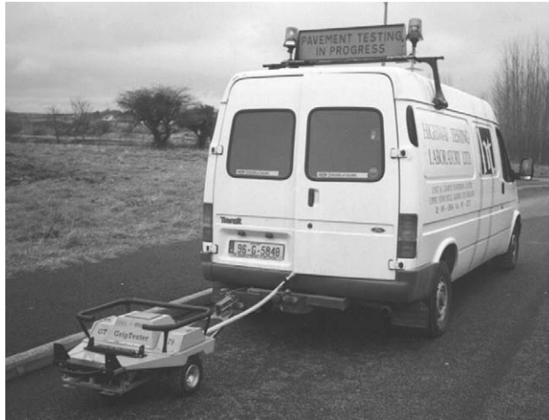
FIGURE 21.4 Griptester in operation.
