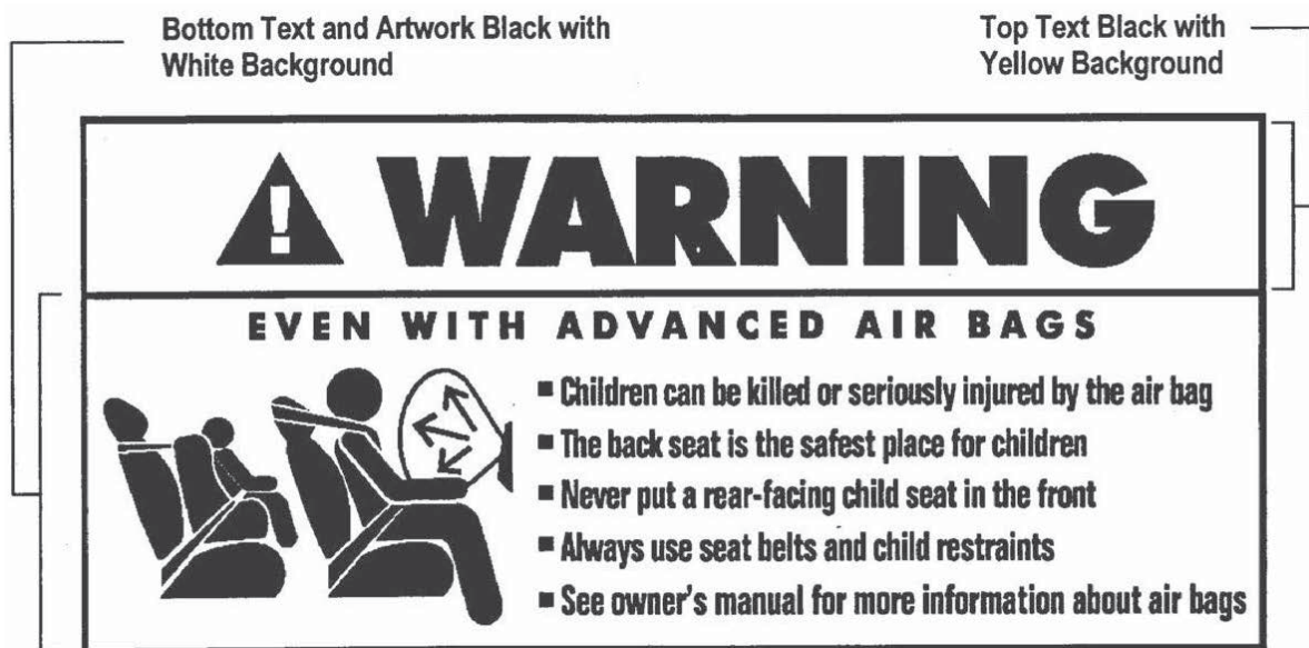
Figure 11. Sun visor Label Visible When Visor in Down Position.
