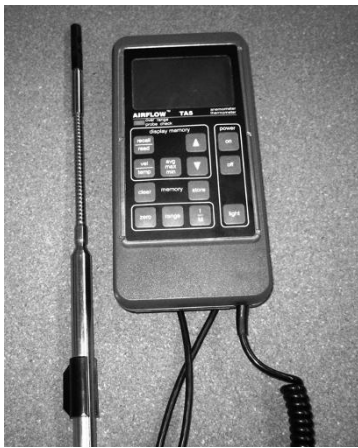
Figure 8.22: A thermal anemometer probe with display unit
