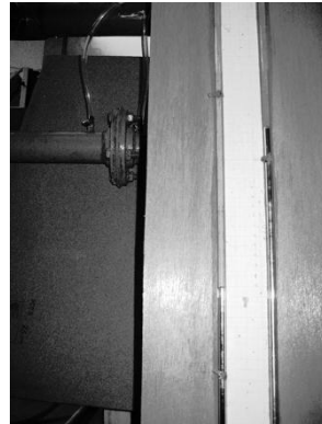
Figure 9.8: Photograph of an orifice plate in use
