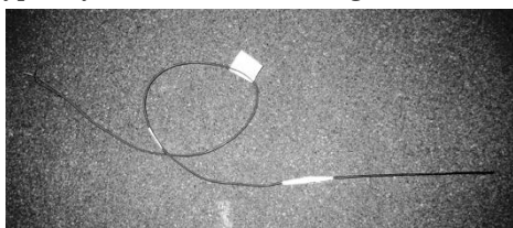
Figure 4.19: Photograph of a K type thermocouple with stainless steel sheath
