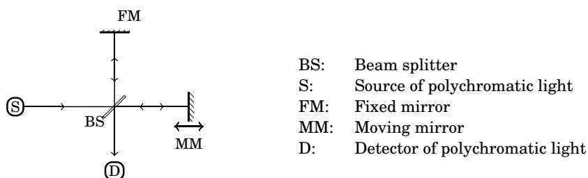
Figure 12.8: Schematic of a Fourier Transform Infrared Spectrometer (FTIR)
