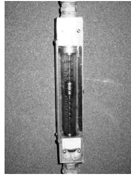
Figure 9.15: Typical Rota meter in the laboratory
