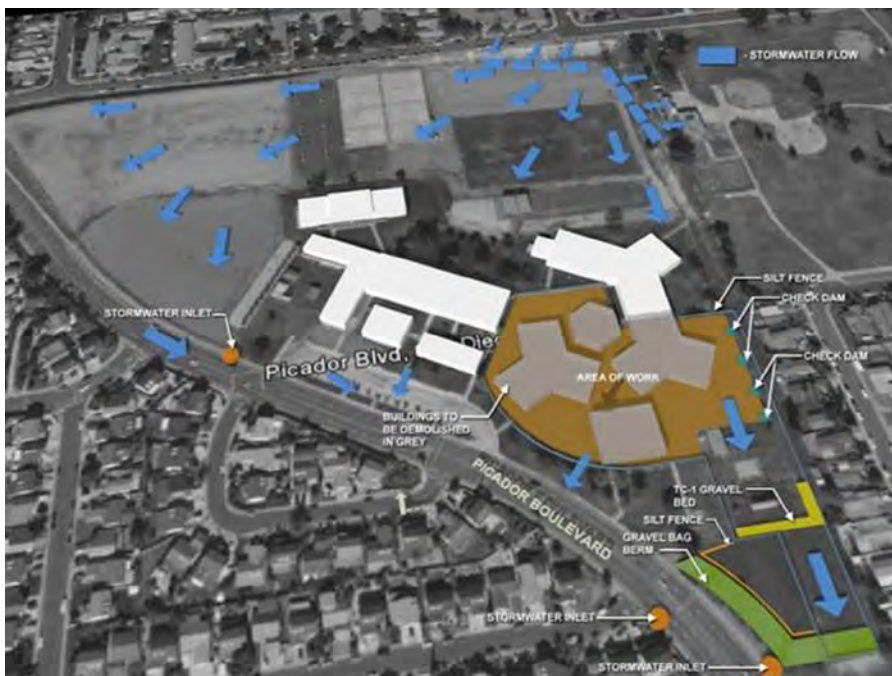
Figure 3.9 Stormwater runoff prevention plan
