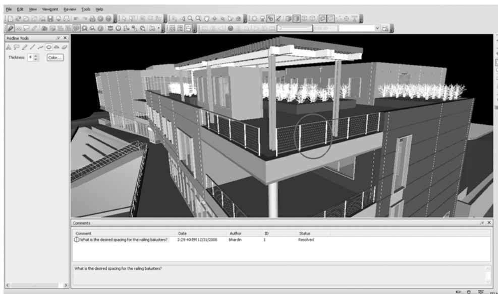
Figure 7.10 Example of Navisworks being used for punch list coordination
