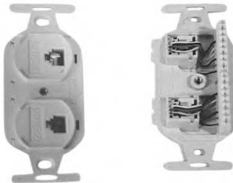
FIXED-DESIGN, DUPLEX, RJ-45 WALL PLATE THAT USES 110 PUNCH-DOWNS
