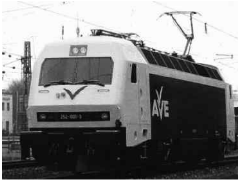
Fig 8.8: RENFE S 252 (5.6 MW; AC 25 kV 50 Hz and DC 3 kV) (Siemens AG, TS)
