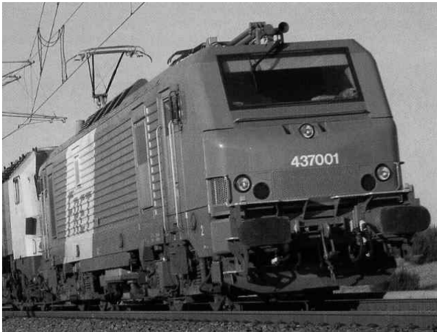
Fig. 7.20: SNCF Class 437 three-system locomotive of the Alstom PRIMA family (type 3U15) (ALSTOM Transports)
