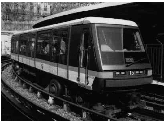
Fig. 12.1: Paris Métro train operating on pressurized rubber-tire wheels in an elevated station [B23]
