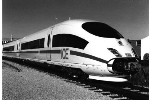
Fig. 1.10: Electric High-Speed Train ICE3 class 403 of DB AG; 1999, 8000 kW, 330kph
