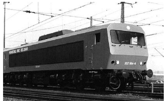
Fig. 1.8: First diesel-electric locomotive with three-phase drive technology DE 2500 by BBC and Henschel 1971; 1840 kW
