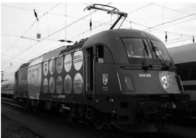
Fig. 7.21: ÖBB Class 1216 ("Taurus") three-system locomotive (cf. Fig. 3.14, too) (Siemens TS)
