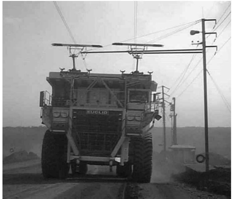
Fig. 12.15: 254-t Haul Truck Euclid-Hitachi R280 under overhead line (Siemens Energy & Automation, Inc.)
