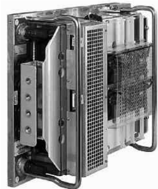
Fig. 6.43: Water-cooled phase building block with 6.5-kV, 600-A IGBTs; U_{dN} = 3\text{ kV} (Siemens AG, A&D)
