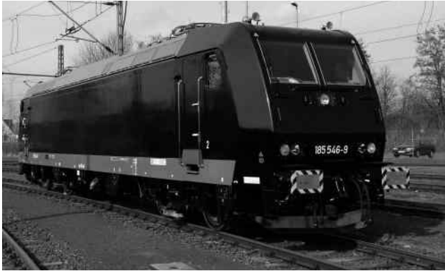
Fig. 7.19: TRAXX F140 AC2 MRCE 185 546 (equivalent to DBAG Class 185.2) Signalling package for German and France (Bombardier Transportation)
