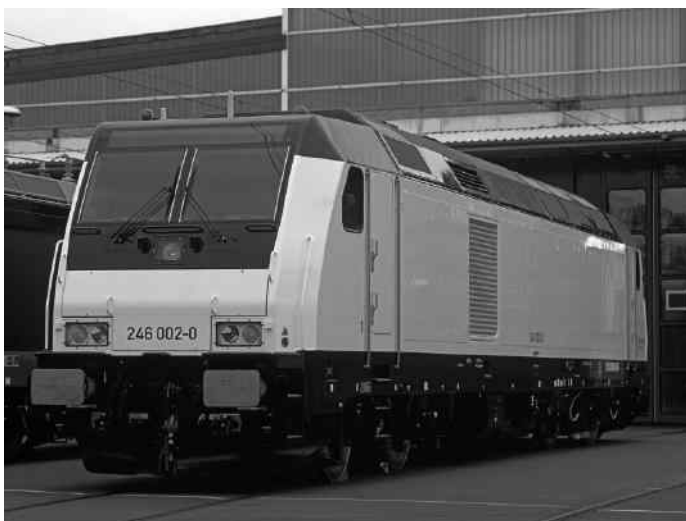
Fig. 9.23: Diesel-electric locomotive TRAXX P160DE, Class 246 LNVG (Bombardier Transportation)
