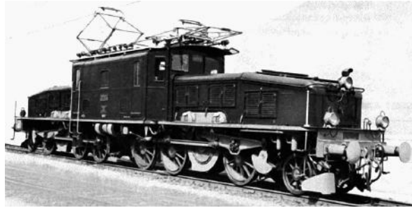
Fig. 1.4: SBB Ce 6/8 II for single-phase AC 15 kV/16 2 / 3 Hz; 1920; 1650 kW
