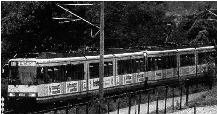
Fig. 10.12: Dual system Light Rapid Transit train GT8-100C/2S on 15-kV, 16 2 / 3 -Hz line (Bombardier Transportation)
