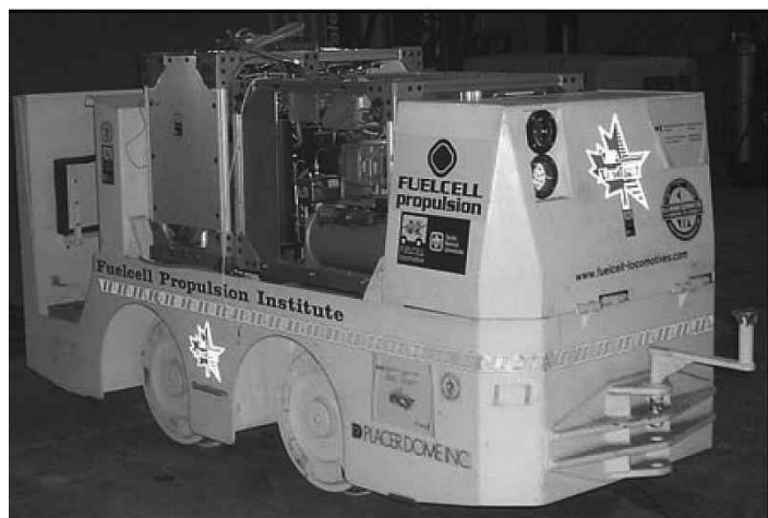
Fig. 10.29: Mining locomotive prototype with PEM fuel-cell stack ( www.fuelcellpropulsion.org )
