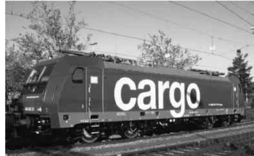
Fig. 8.12: SBB Class Re 484 with 6.5-kV IGBT inverters operated with the 4q-C as pre-chopper in 3-kV DC mode (Bombardier Transp.)
