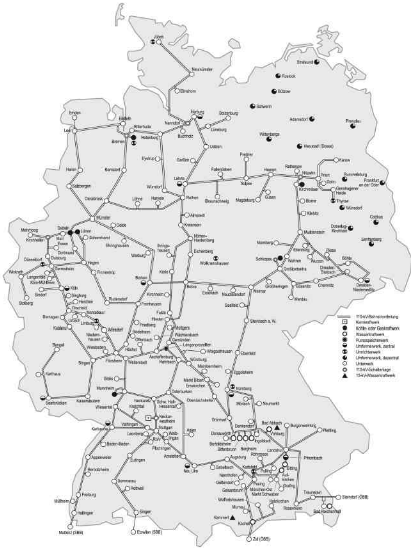
Fig. 13.2: 110-kV railway interconnected mains of DB Energie GmbH, as of 01.01.2007 [177]
