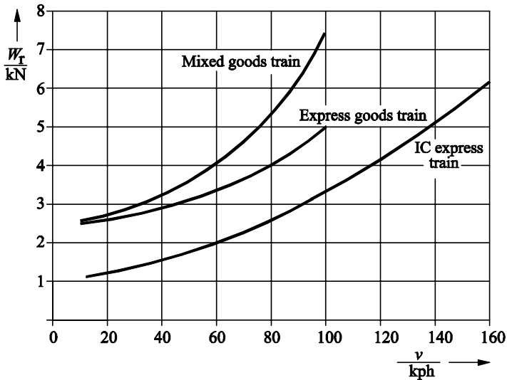
Fig. 2.13: Train rolling resistance according to formulas used at DB (IC: 16 coaches)
