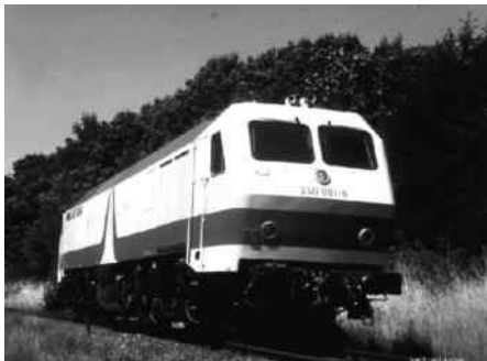
Fig. 9.18: Locomotive DE 1024 ABB-MaK P_D = 2,650 kW, v_{max} = 160 kph (Bombardier Transportation)
