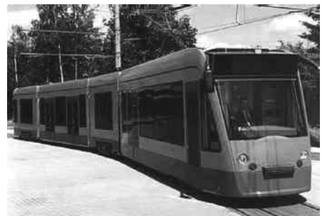
Fig. 10.23: 100 % low-floor multi-joint tram Combino (DÜWAG-Siemens)
