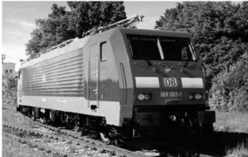
Fig. 8.11: DBAG Class 189, with 6.5-kV IGBT inverters operated directly off the 3-kV DC mains (Siemens AG, TS)
