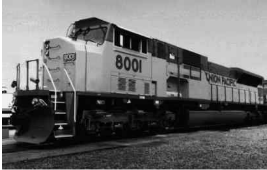
Fig. 9.20: Diesel-electric locomotive SD 90 MAC of Union Pacific RR, by GM-EMD and Siemens (Siemens AG, TS)
