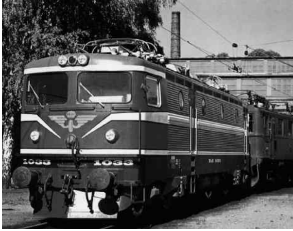
Fig. 7.2: Locomotive Rc2 of SJ, with thyristor phase-angle control
