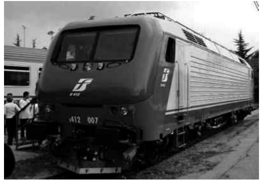
Fig. 8.9: FS Italia Class E 412 (6 MW, AC 15 kV/16 2 / 3 Hz; 1.5 and 3 kV) (Bombardier Transportation)
