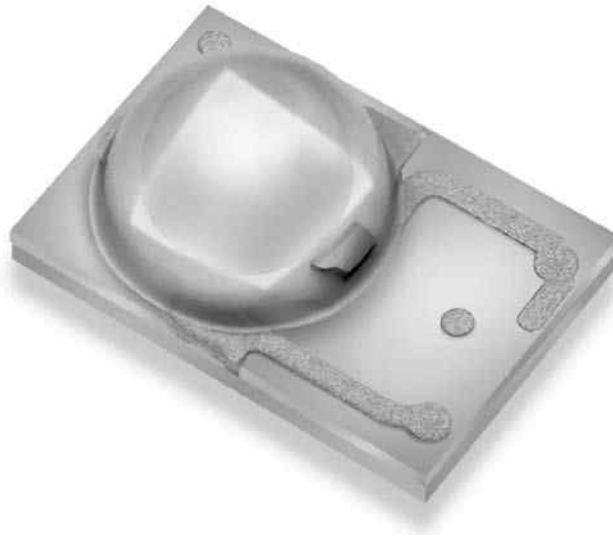
Figure 5.28 Photograph of high-power LED capable of over 300 lumens output. The rectangular ceramic plate is designed for ease of mounting and heatsinking. Specific applications of these LEDs include street lighting, retail lighting and automobile headlights. Reproduced from www.luxeon.com . Copyright (2011) LUXEON
