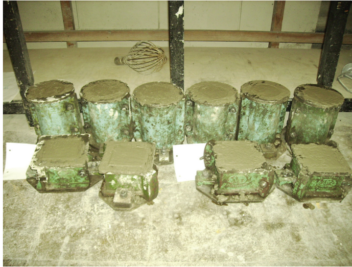
FIGURE 22.12 Filled Cube and Cylinder Moulds
