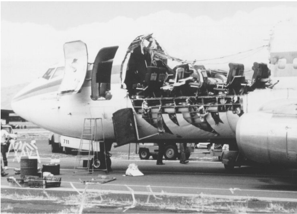
Figure 1.11 Fuselage failure in a passenger jet that occurred in 1988. (Photo courtesy of J. F. Wildey II, National Transportation Safety Board, Washington, DC; see [NTSB 89] for more detail.)
