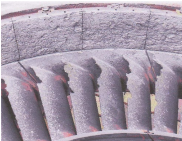
Figure 1.8 Solid particle erosion. Source: Wilcox et al. (2010).
