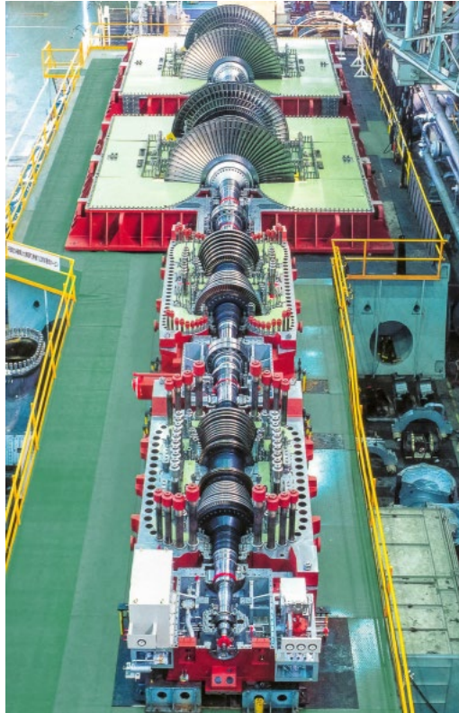
Figure 1.3 700 MW ST Hekinan Unit 3, Chubu Electric Power Co. Source: Reproduced by permission of Mitsubishi Hitachi Power Systems America, Inc.
