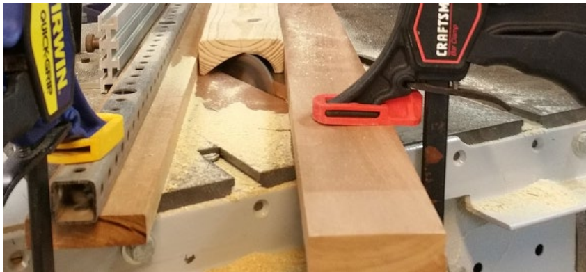
Figure 12.8 Asymmetric cove on the table saw.
