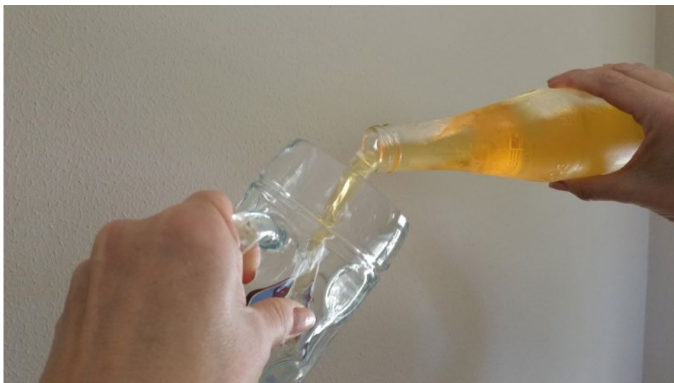
Figure 9.7 Pouring with Froude number greater than 0.3.
