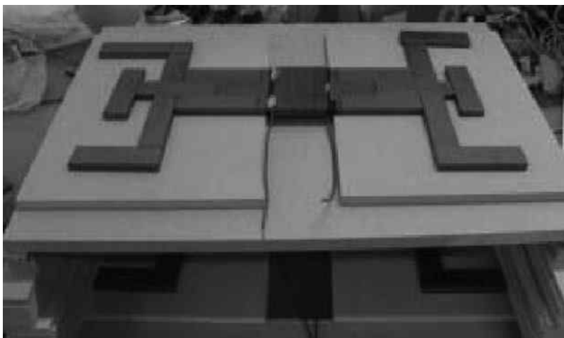
Figure 10.27 The double-sided coils used by the Auckland team. © 2015 IEEE. Reprinted with permission from Choi et al. (2015c)
