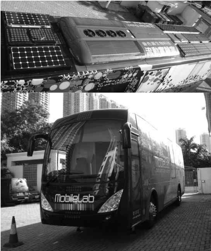
Figure 5.12 The roof of the mobile laboratory with PV (above) and the outlook of the mobile laboratory (below). (Photo courtesy: Dr. William MAK)
