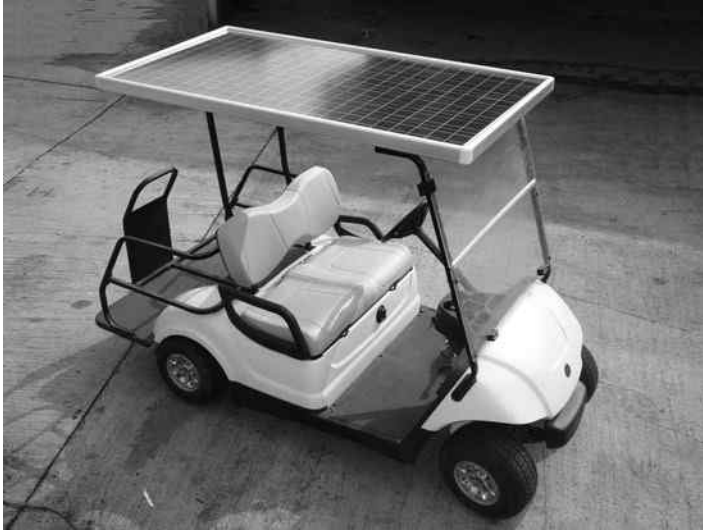
Figure 5.10 Putting a PV module as the roof of a golf-cart. (Photo courtesy: Mr. Jackson FUNG)
