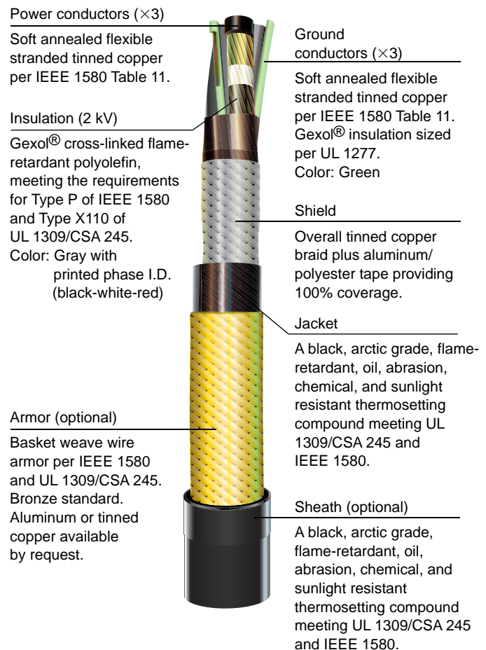
Figure 10-17 VFD shielded power cable.
