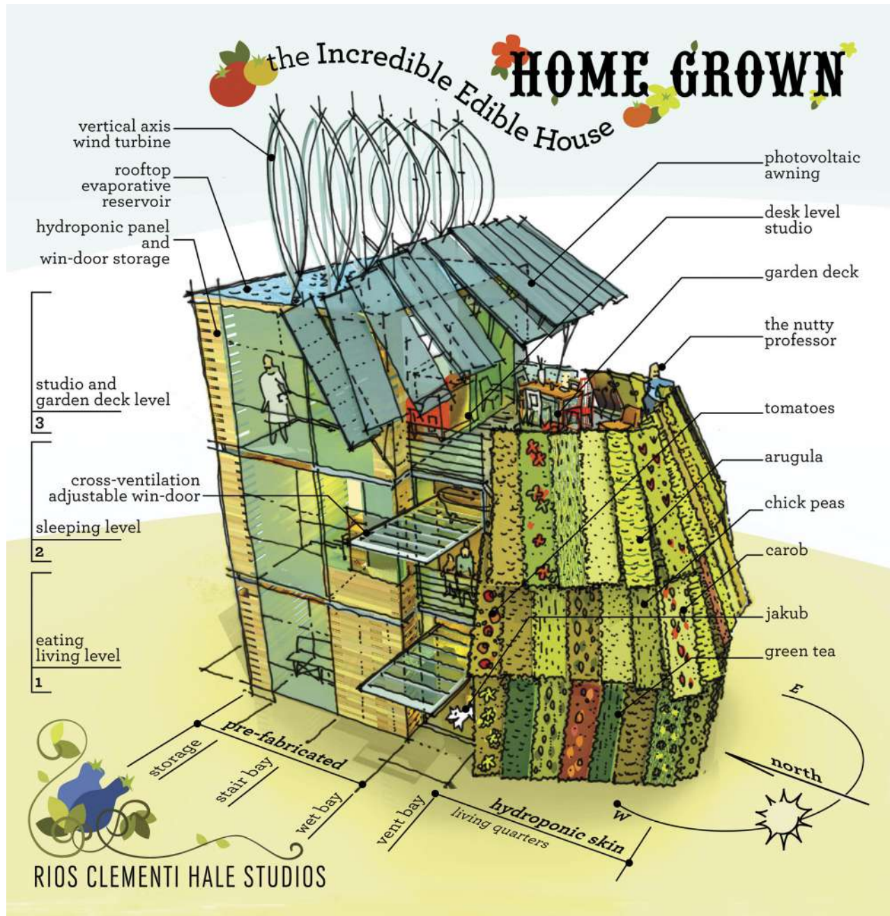
Figure 4.19 The Incredible Edible House and its components to meet a family of four's food and sustainable living needs.
