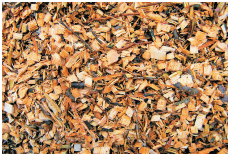
FIGURE 15-13 Wood chips for biomass combustion.
