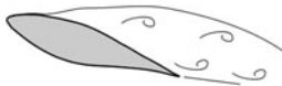
Fig. 33 The process of dynamic stall involves several distinct stages, but the shedding of a concentrated vortical disturbance from the leading edge of the airfoil is a distinguishing feature of the phenomenon
