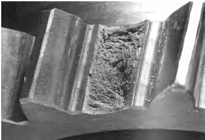
Fig. 7.2. Brittle overload failure of a helical-cut spur gear [7.40]
