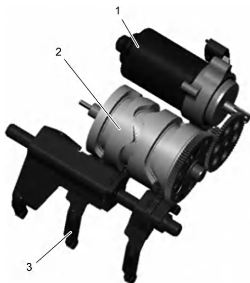
Fig. 12.14. Electromechanical activation of the sliding sleeves of the gearbox Getrag 431.
