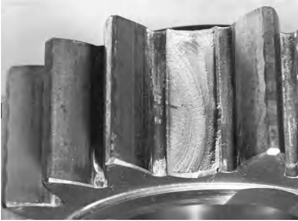
Fig. 7.3. Vibration fatigue failure of a straight spur gear [7.40]
