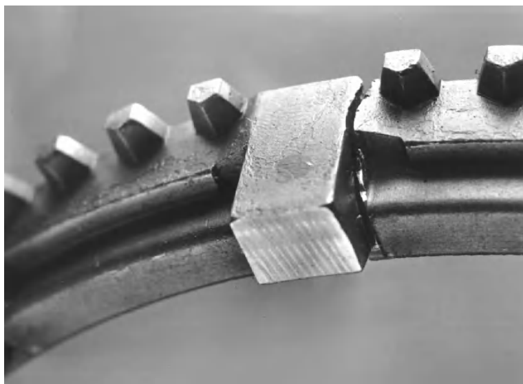
Fig. 9.17. Damage to the synchronizer ring caused by torsional vibration, fracture at the stop boss
