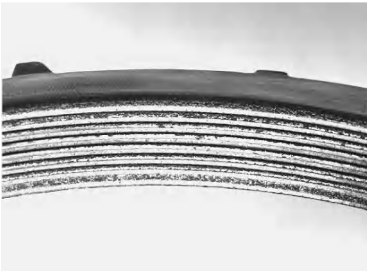
Fig. 9.19. Increased wear at the molybdenum friction surface of a commercial vehicle synchronizer ring caused by thermal overload
