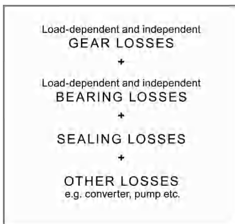
Fig. 2.32. Composition of losses in vehicle gearboxes
