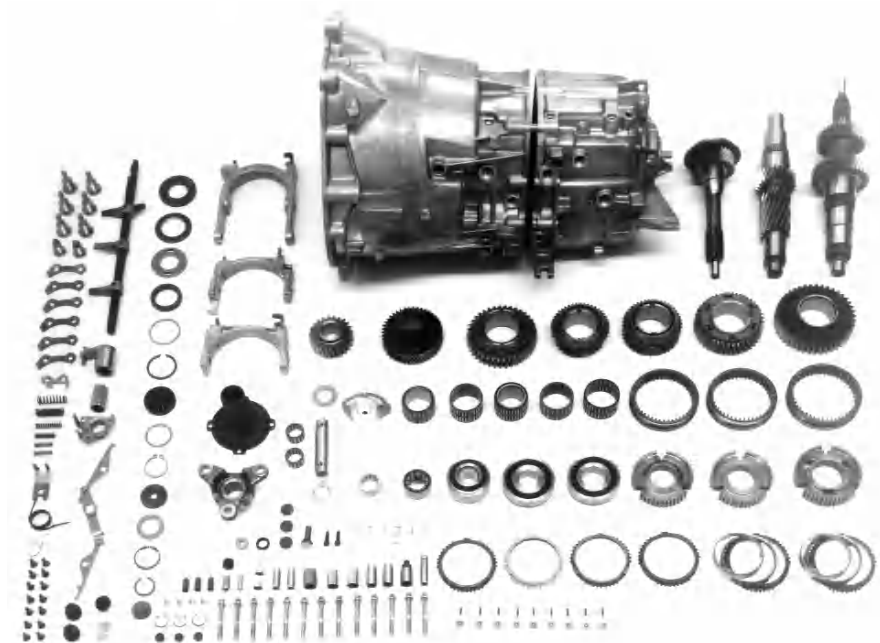
Fig. 12.4. Individual parts of the 5-speed manual passenger car gearbox ZF S 5-31
