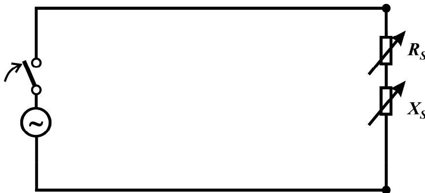
Fig. 13.1. Alternating voltage line with active R_S and reactive X_S load at receiving end.
