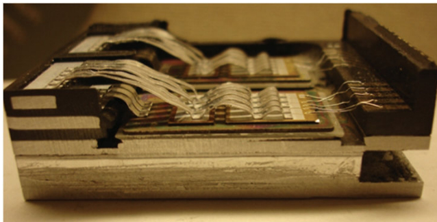
Figure 11.3 Views of boost and inverter silicon for the 2010 Toyota Prius [1]. (Courtesy of Oak Ridge National Laboratory, US Dept. of Energy.)
