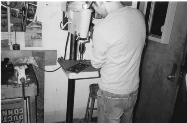
FIGURE 11.11 Student fabricating a new truss plate in Engineering Machine Shop.
