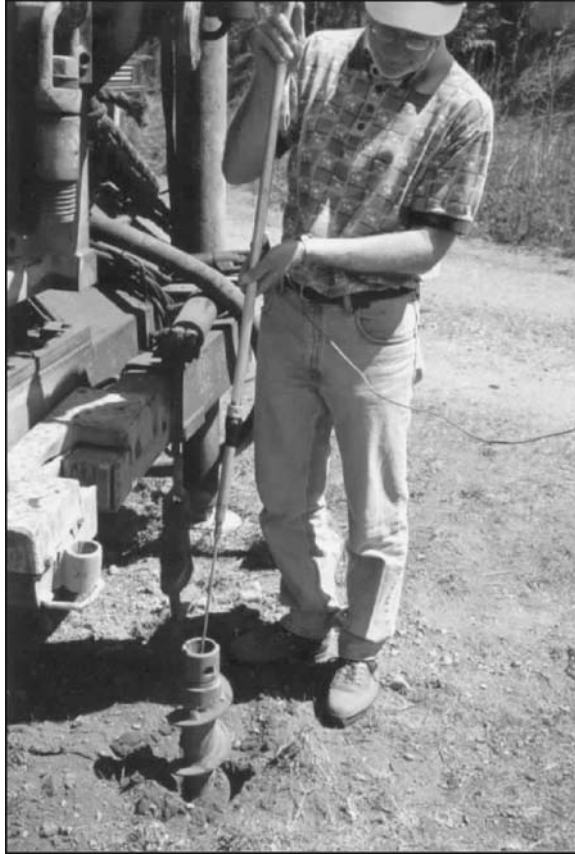
FIGURE 14-86 Thermal probe being inserted into an auger during geotechnical testing.
