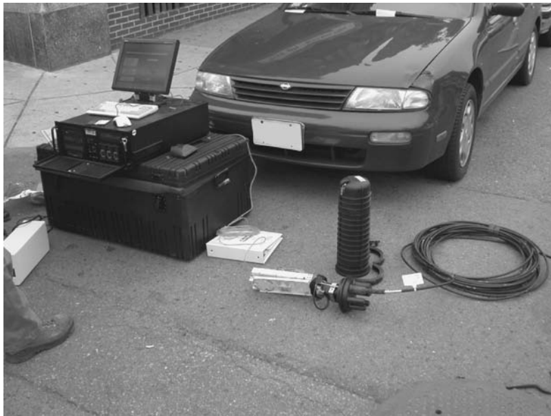
FIGURE 14-84 Distributed temperature system and fiber being used in the field to measure cable temperatures.
