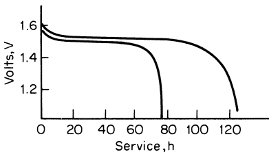
FIGURE 11-38 Discharge curves of zinc-silver oxide cells.
