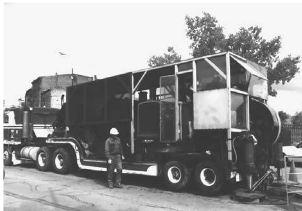
FIGURE 14-92 Pulling winch trailer.
