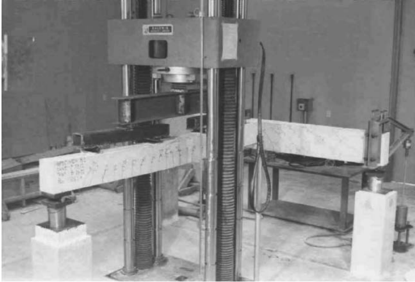
Figure 7.17 Testing of T-shaped specimen
