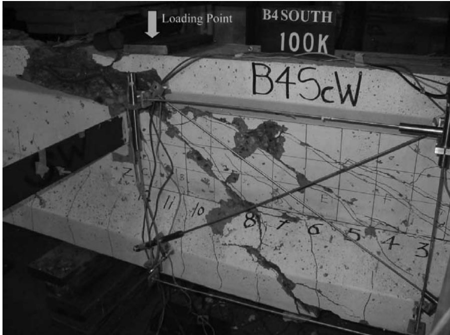
Figure 8.13 Beam B4 showing 45° failure crack in flexural-shear failure zone
