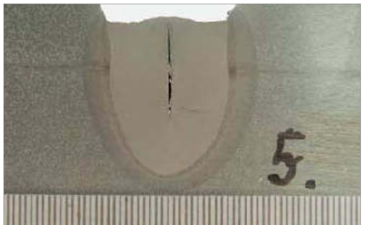
Weld depth to width ratio > 1 and relatively large amount of impurities in base material (S, P, Nb).
