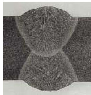
Two-sided square edge with cored wire
