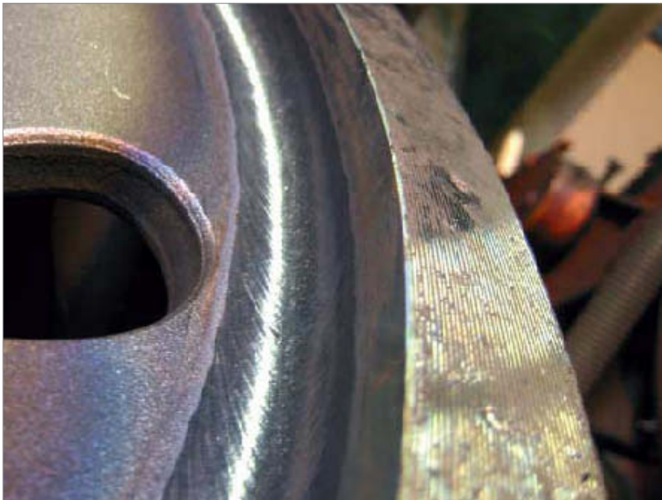
Downhand (PA/1F) fillet weld showing perfect wetting and smooth finish.
