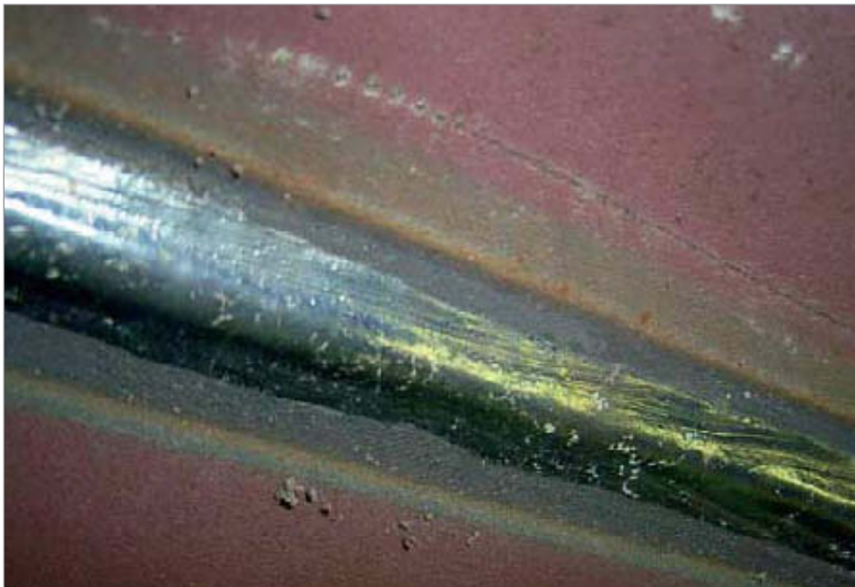
Underside of one-sided joint welded using OK Flux 10.69 backing flux.
