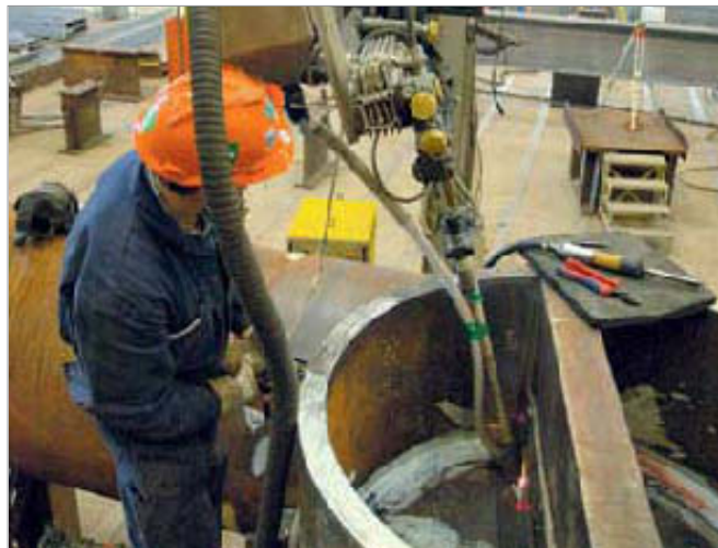
Deposition rate comparison OK Tubrod 15.00S and OK Autrod 12.20 / OK Flux 10.71.
