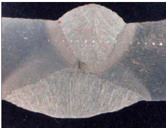
Insufficient penetration and excessive reinforcement; also misaligned.
