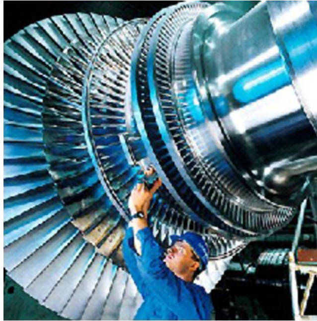
Figure 6.20 A turbine rotor fixed with a diaphragms and blades. Source: STEAM TURBINE. Wikipedia the Free Encyclopedia.
