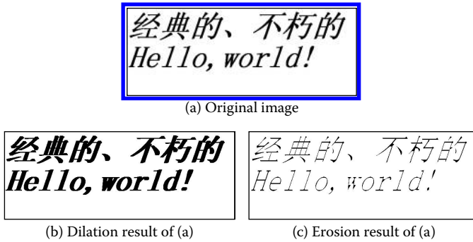
FIGURE 5.6 The results of binary dilation and erosion operations: (a) the original image, (b) dilation result of (a), and (c) erosion result of (a).
