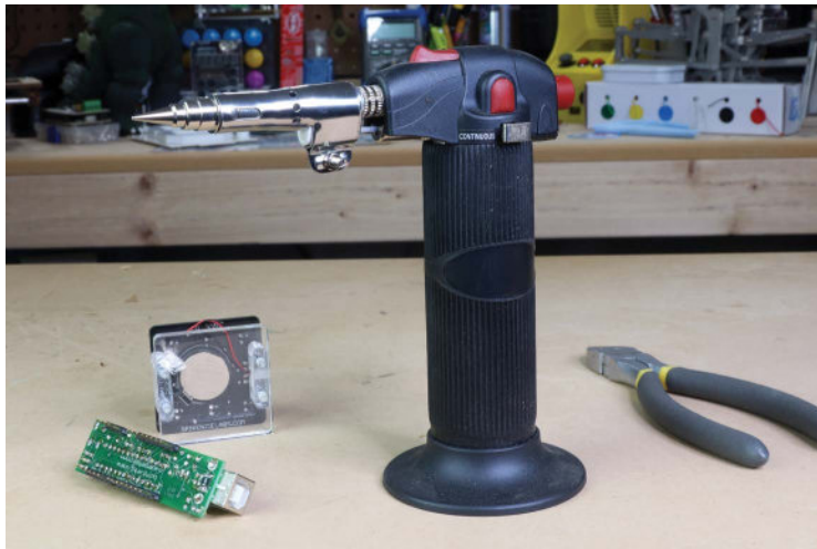
FIGURE 2-14: Gas-fueled soldering iron
