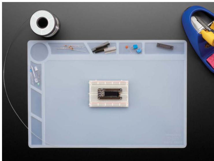
FIGURE 5-5: Insulated silicone rework mat IMAGE COURTESY OF ADAFRUIT INDUSTRIES, CC BY-NC-SA 2.0.
