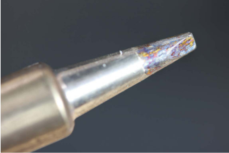
FIGURE 3-3: A dirty soldering iron
