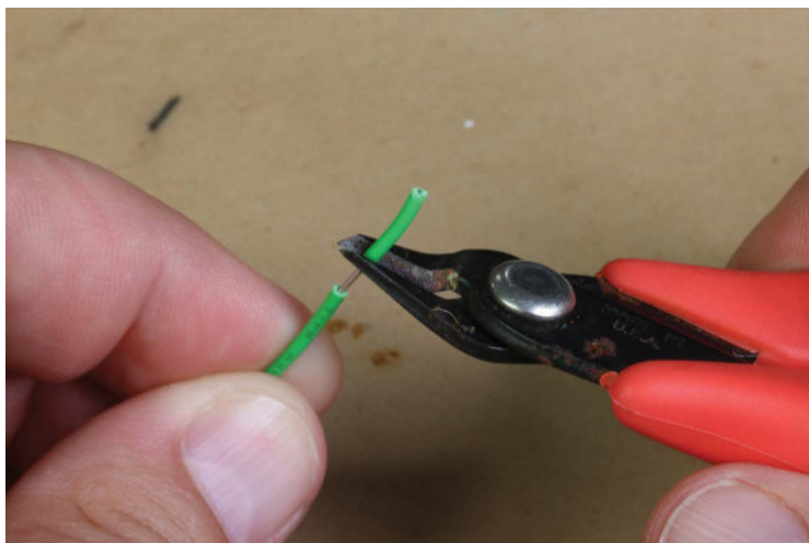
FIGURE 2-21: Using flush cutters to strip solid core wire
