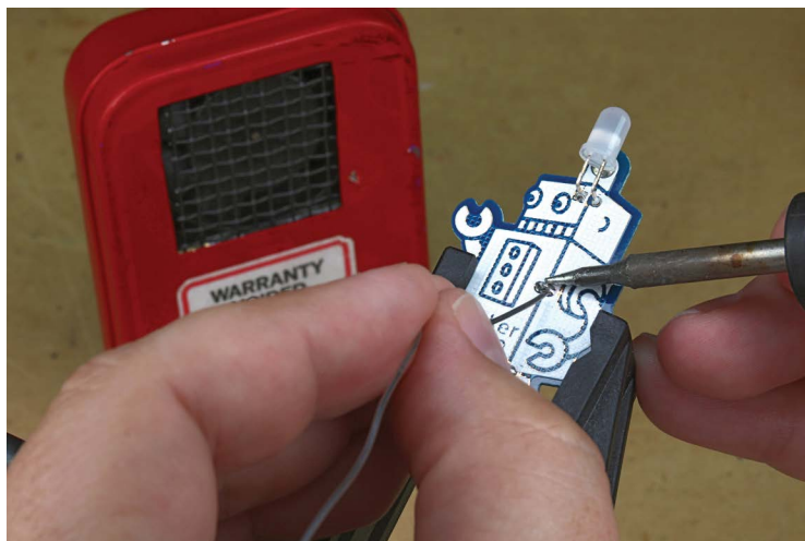
FIGURE 1-1: Depositing solder on a “learn to solder” pin designed by the author
