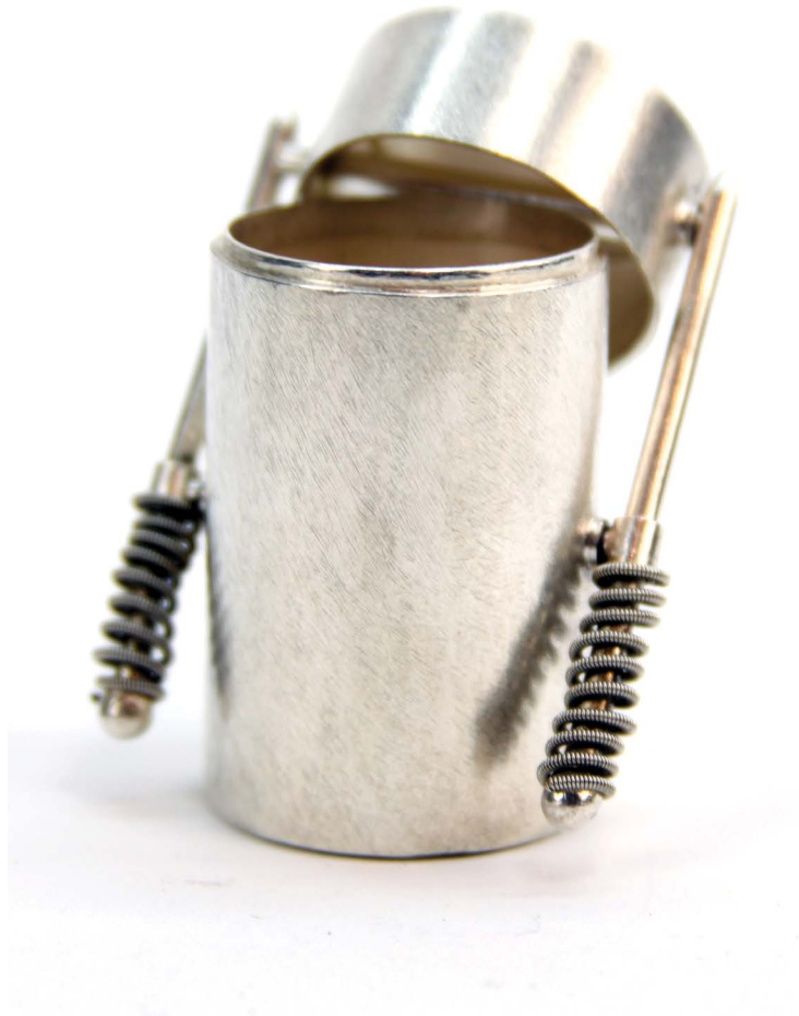
FIGURE 1-4: A spring-loaded box created with silver soldering made by the author
