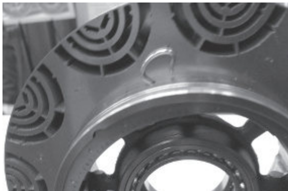
Figure 12.6: Rotor of Chevrolet Volt ferrite motor that has four layers.
