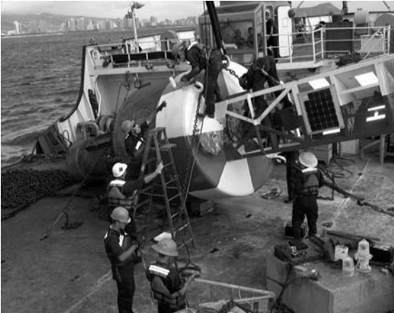
Figure 2.19 Aids to Navigation: Honolulu, HI – Coast Guard Cutter Walnut (WLB 205) deck crew paints the 18 000-lb. Hotel buoy. (Photo courtesy of Sarah Foster-Snell).
