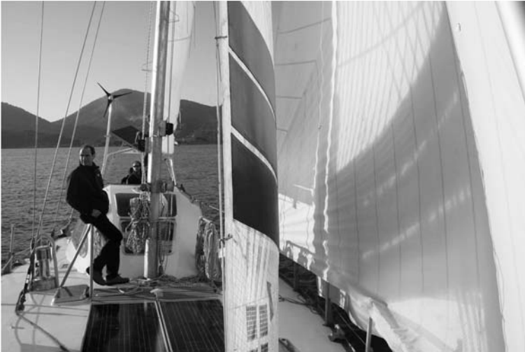
Figure 4.22 The ship currently navigates in Italy's seas using a hybrid motor (diesel + electric) with solar electricity being produced by either Si or organic (polymer with carbon nanotubes) photovoltaic thin films. (Photo courtesy: Michelangelo Calamai & Figli).
