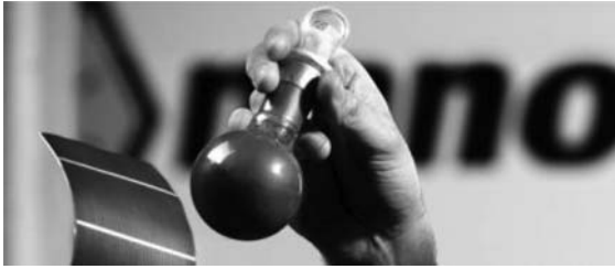
Figure 3.16 Nanosolar's nanostructure CIGS ink. (Photo courtesy: Nanosolar).
