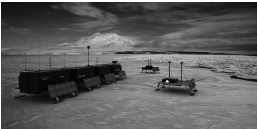
Figure 1.16 Testing of thin-film solar panels in the Antarctic. (Photo Courtesy: Nanosolar).
