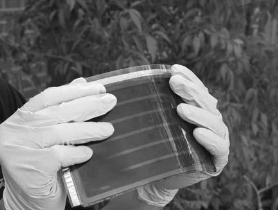
Figure 5.11 A flexible, plastic dye solar module manufactured by Peccell Technologies.
