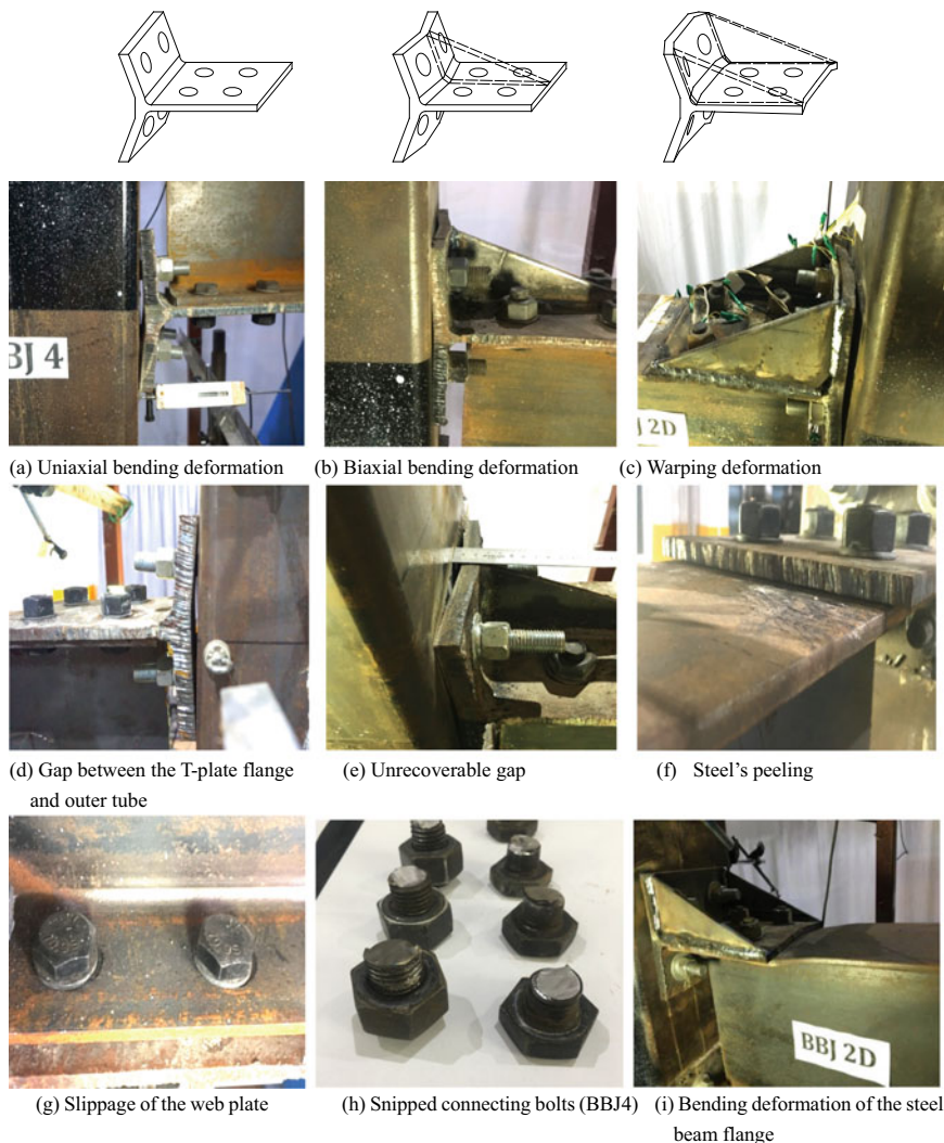
Fig. 9.4 Failure process photos
