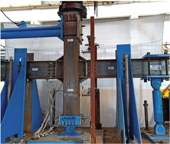
Fig. 8.2 Test setup of the anchored web joint
