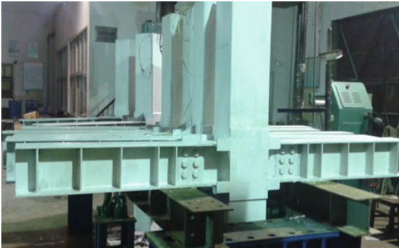
Fig. 6.4 Details of the square CFST column-to-beam joint (SBJ4-1)
