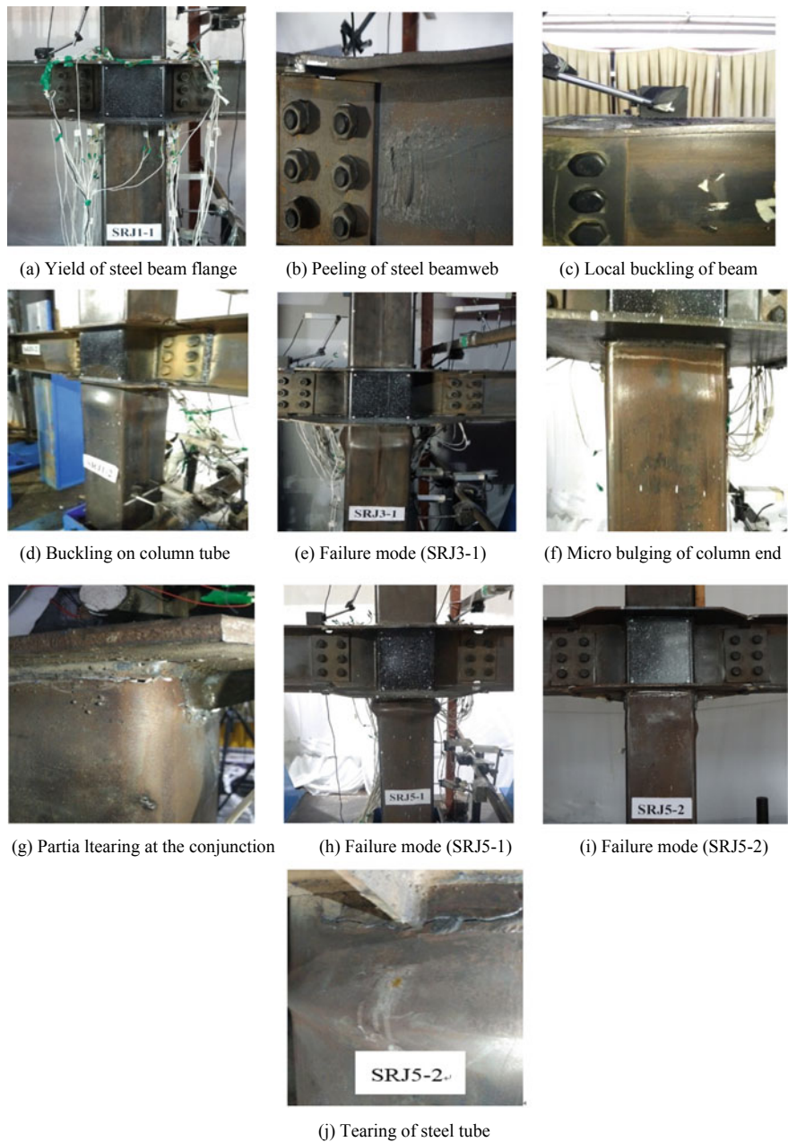
Fig. 7.6 Failure phenomena of the joint specimens
