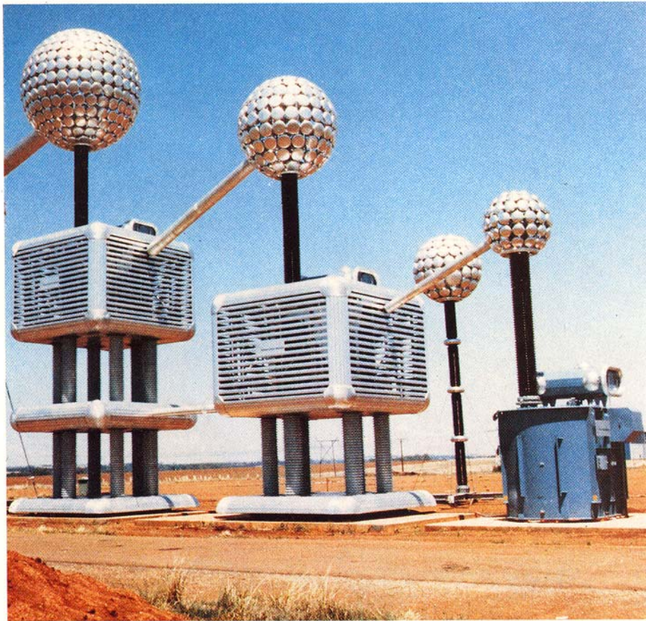
Three-stage cascade transformer 3 x 600 kV, 2 A cont. outdoor type with AC voltage divider 1500 kV
