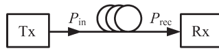
Figure 7.1 A simple fiber-optic system consisting of a transmitter, a receiver, and an optical fiber.
