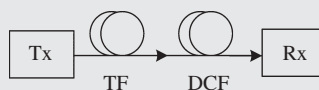
Figure 2.39 Fiber-optic system consisting of TF and DCF. TF = transmission fiber, DCF = dispersion-compensating fiber, Tx = transmitter, and Rx = receiver.
