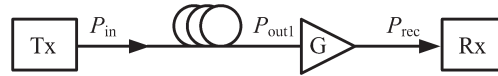
Figure 7.5 A fiber-optic system consisting of a transmitter, a fiber, an amplifier, and a receiver.
