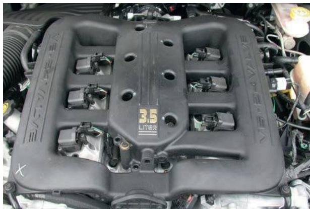
Figure 2.312 Six direct ignition coils in position
