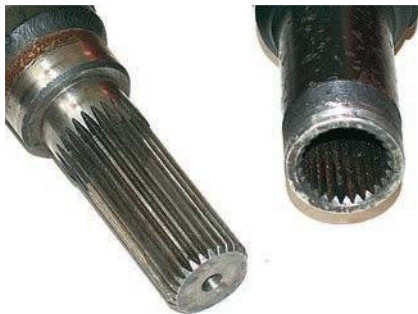
Figure 5.87 A splined joint connects to the gearbox
