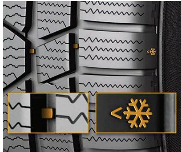
Figure 4.152 Once the tread is worn down to 4 mm, the Winter Indicator becomes level with the surface of the tread pattern, indicating that the tyre has reached its limit of winter suitability. (Source: Continental)
