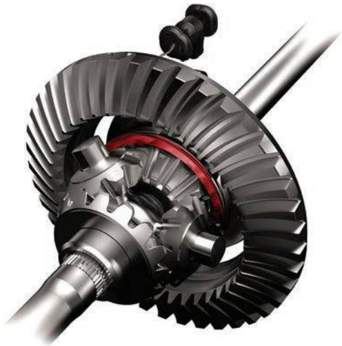
Figure 5.116 Differential locking mechanism [highlighted]. (Source: Ford Media)
