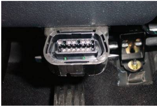
Figure 3.33 DLC socket – pin 6 is CAN-high and pin 14 is CAN-low
