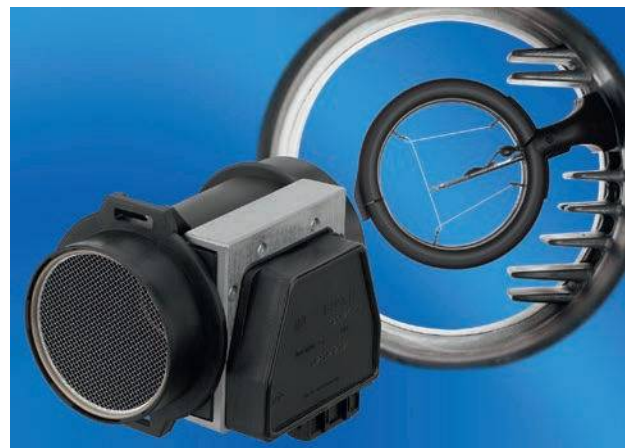
Figure 2.243 Hot wire/film air flow meter
