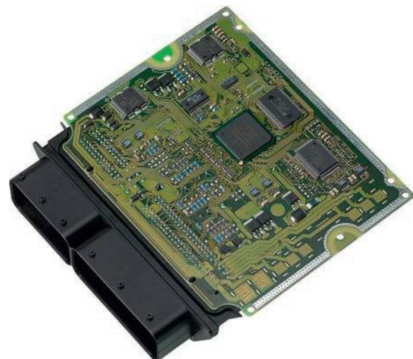
Figure 2.235 Inside an electronic control unit (ECU)
