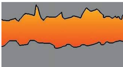
Figure 2.116 Boundary lubrication uses the oil to prevent two rough surfaces from touching
