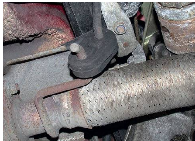
Figure 2.197 Flexible mountings (sometimes called pig noses)
