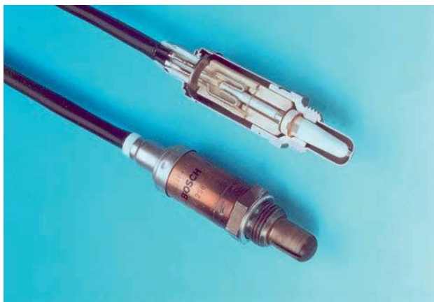
Figure 2.249 Construction of a zirconia type lambda sensor
