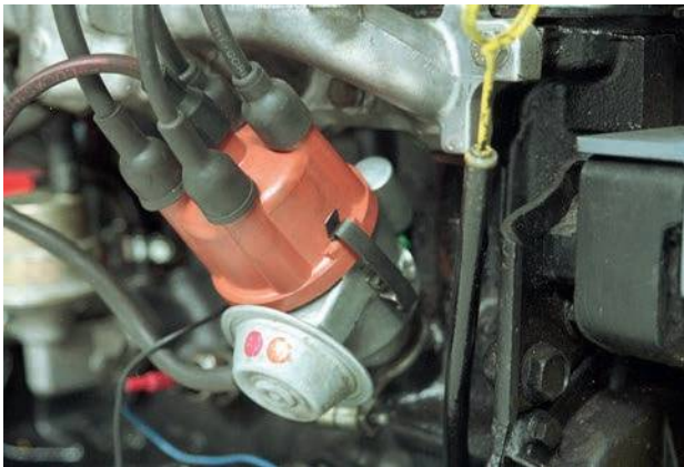
Figure 2.302 Traditional system using a distributor
