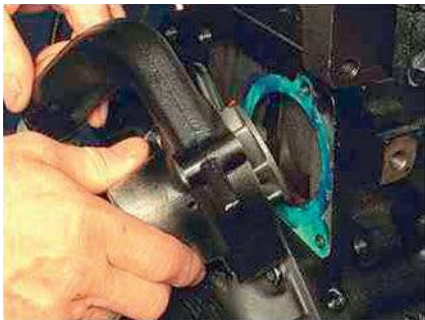
Figure 2.163 Water pump in water jacket
