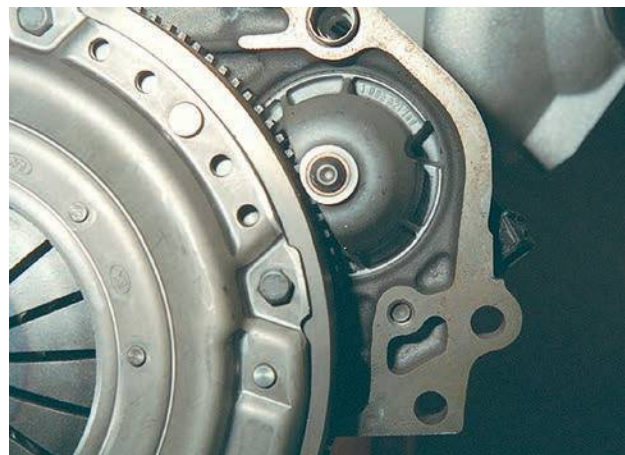
Figure 3.62 Starter in position to mesh with a ring gear on the engine flywheel
