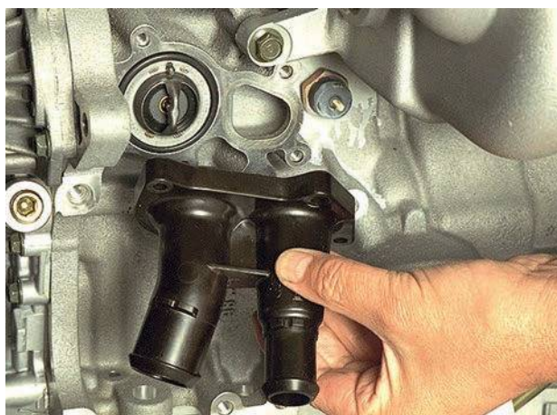
Figure 2.145 Engine coolant ports with a thermostat in position
