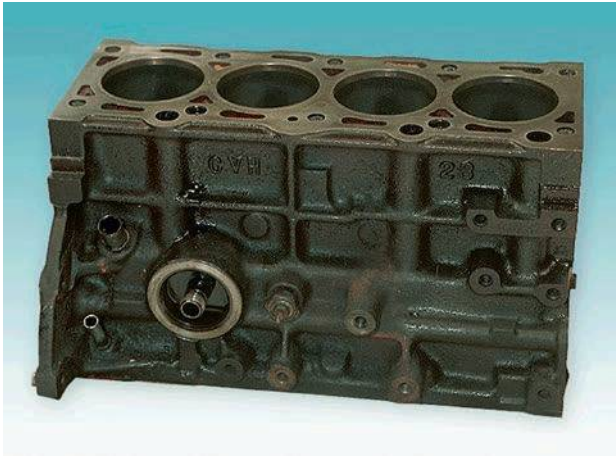
Figure 2.52 Cast iron engine block
