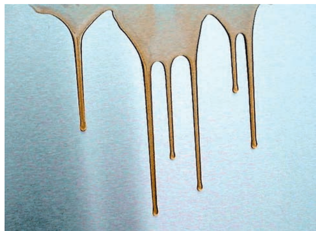
Figure 2.115 Viscosity is the resistance to flow
