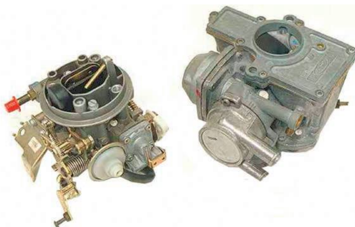
Figure 2.225 Fixed-choke (left) and variable-choke (right) carburetors
