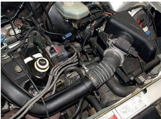
Figure 2.185 Air supply components
