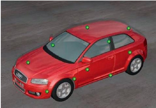
Figure 1.16 Body components (clockwise from the left): 1, bonnet (hood); 2, windscreen; 3, roof; 4, tailgate; 5, post; 6, rear quarter; 7, sill; 8, door; 9, front wing; 10, front bumper/trim
