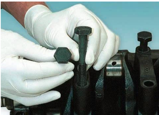
Figure 2.57 Main bearing bolts
