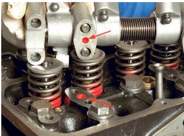
Figure 2.122 Oil drillings for the valve gear
