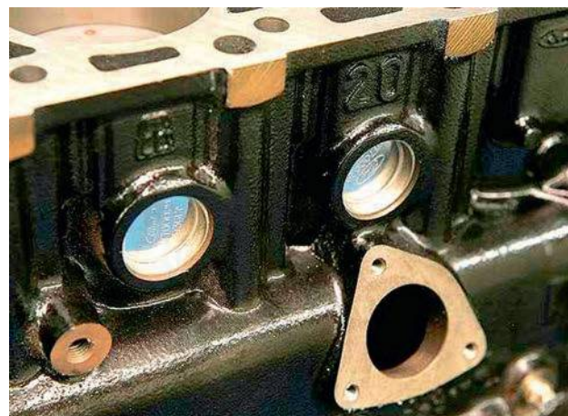
Figure 2.142 Engine block water jacket and core plugs
