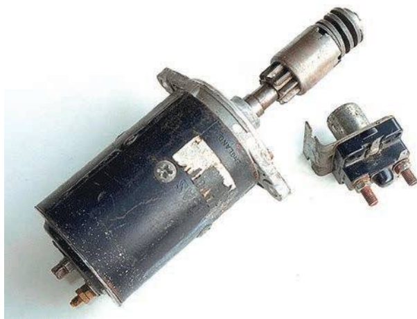
Figure 3.58 Inertia motors with a solenoid switch were used on older cars but have now been replaced by the pre-engaged drive
