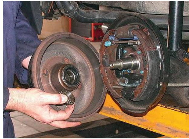
Figure 5.100 Rear hub (dead axle) with taper bearing
