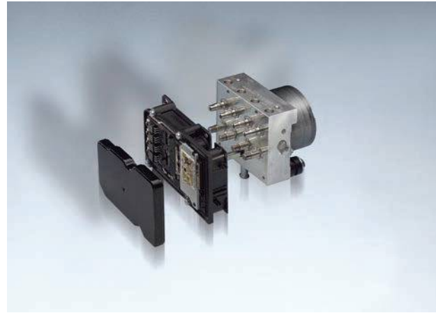
Figure 4.172 ABS 8 exploded view showing the ECU and eight 2/2-way solenoid valves (two hydraulic positions and two hydraulic connections)
