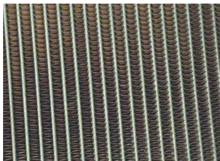
Figure 2.136 Elements of a radiator; a key component in the cooling system
