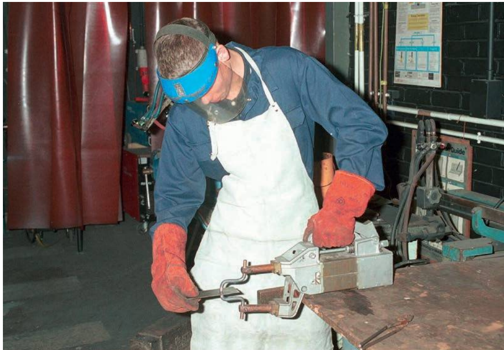
Figure 1.39 Protective clothing for spot welding
