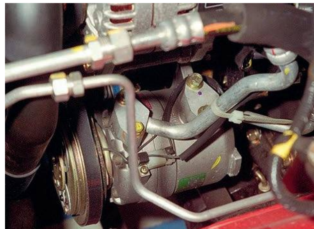
Figure 3.164 Air conditioning system compressor in place
