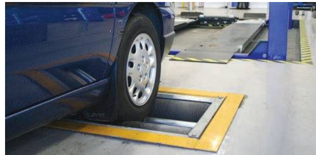
Figure 4.167 Brake roller testing. (Source: Tecalemit)
