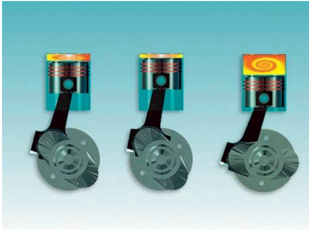
Figure 2.23 Ideal, retarded and advanced ignition point
