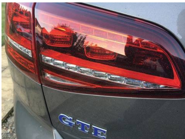
Figure 3.91 Stop and reverse lights form part of the rear light cluster
