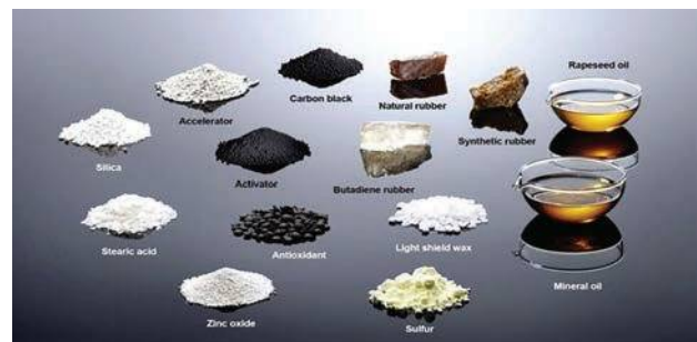
Figure 4.140 Overview of tyre materials. (Source: Continental)
