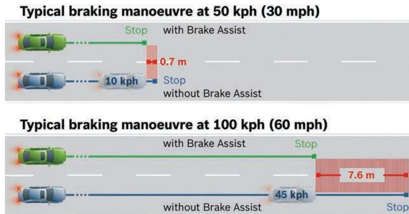
Figure 4.123 Shorter braking distance using EHB. (Source: Bosch Media)
