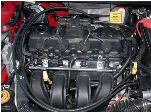
Figure 2.307 Distributorless ignition coil in position
