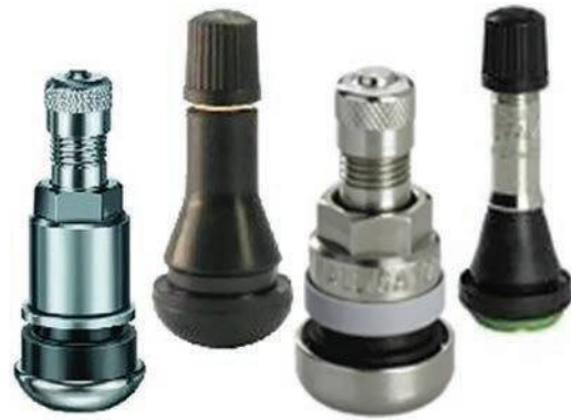
Figure 4.139 Various 'tubeless' valves
