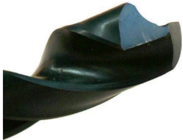
Figure 1.83 Cutting edges and flutes of a drill bit
