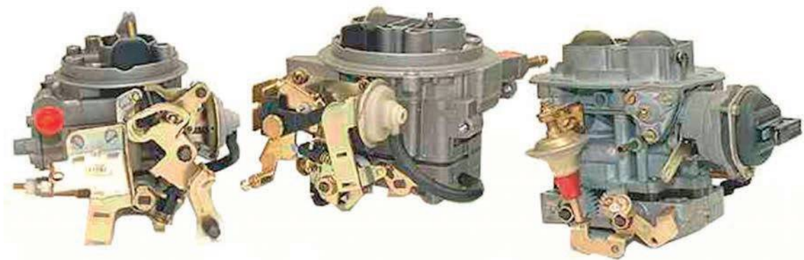
Figure 2.224 Single-choke (left) and twin-choke (middle and right) carburettors
