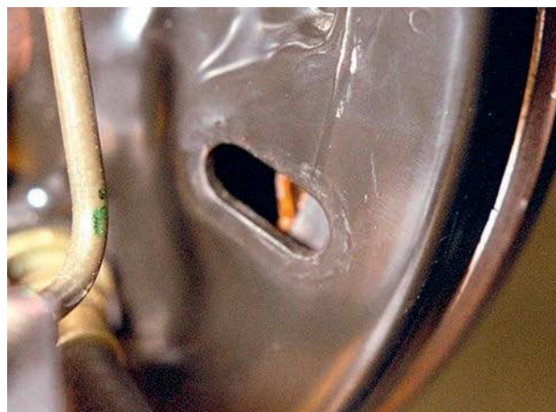
Figure 4.96 Drum brake adjustment hole
