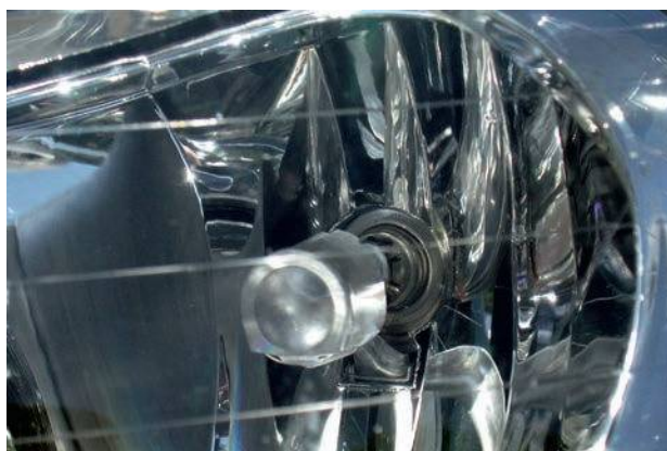
Figure 3.89 Headlights with a clear lens and complex reflector
