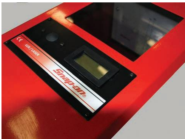
Figure 3.90 Beam setter in use
