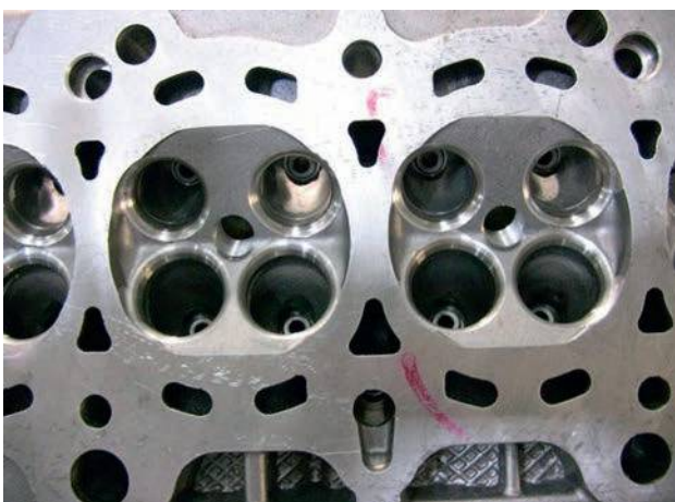
Figure 2.92 Hardened seats in an aluminium head
