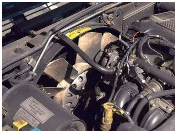
Figure 2.169 Viscous-fan hub on an earlier engine
