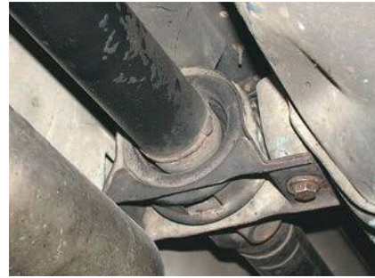
Figure 5.88 This rubber mounted bearing prevents propshaft whip
