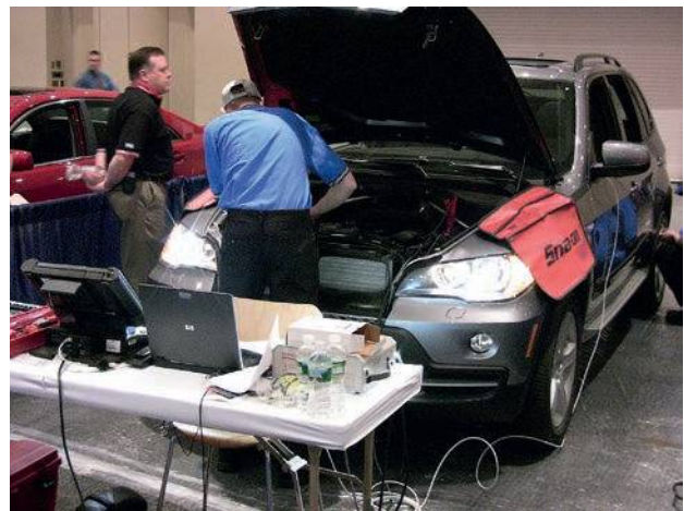
Figure 1.99 Bodywork protection in use during repairs
