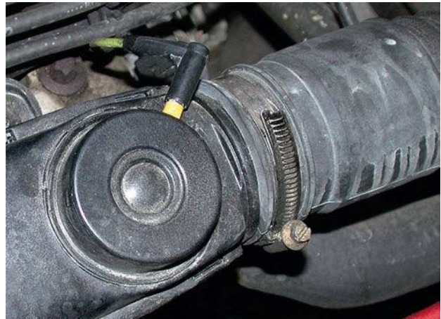
Figure 2.182 Air temperature control valve
