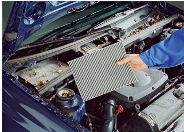
Figure 2.173 Heater intake with pollen filter
