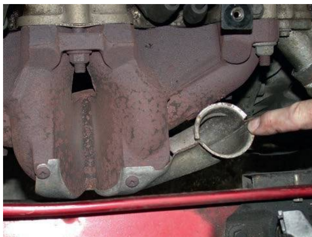
Figure 2.189 Pick-up for hot air on an exhaust manifold
