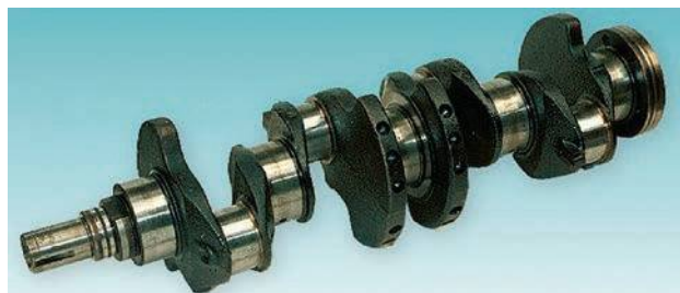
Figure 2.75 Crankshaft: 1–5 main journals
