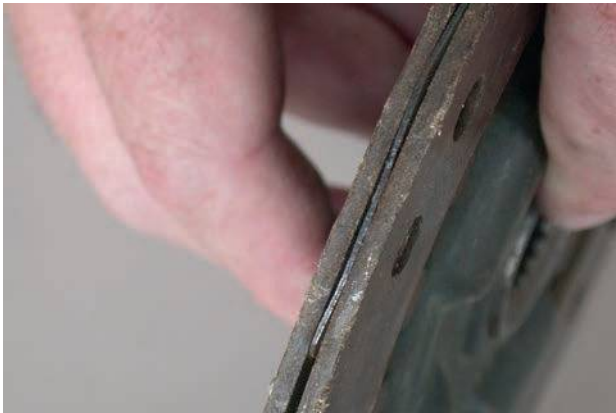
Figure 5.11 Wave springs eliminate chatter
