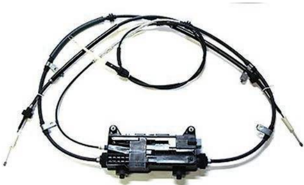
Figure 4.165 Cable pull system. (Source: Land Rover)
