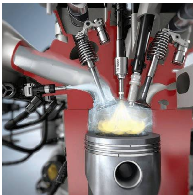
Figure 2.322 Water injection can produce extra boost for the turbocharged engine. (Source: Bosch Media)
