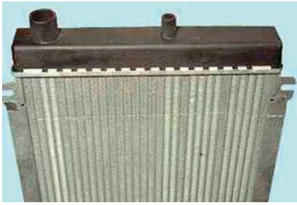
Figure 2.161 Aluminium and plastic radiator
