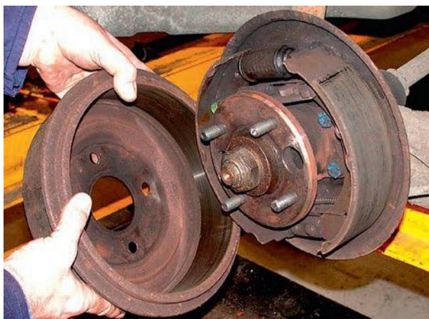
Figure 4.94 Brake drum being removed
