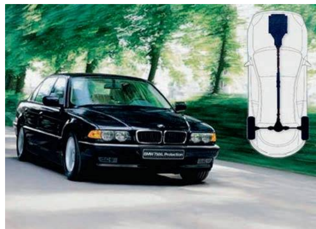
Figure 1.2 Front-engine, rear-wheel drive
