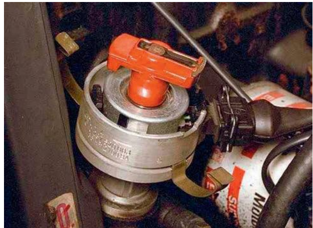
Figure 2.240 Distributor for engine speed sensing on early systems
