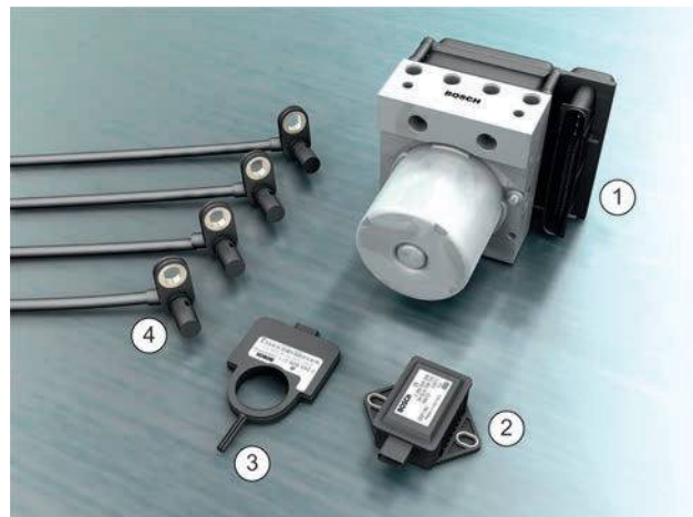
Figure 4.125 Components of an electronic stability program (ESP): 1, Anti-lock braking system and traction control modulator with built-in electronic control; 2, position sensor; 3, steering sensor; 4, wheel speed sensors
