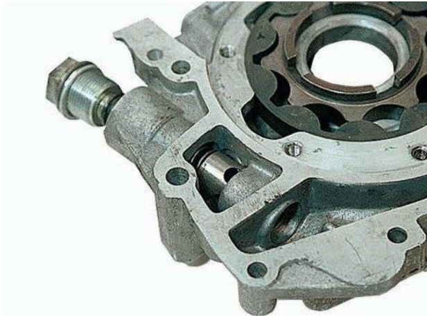
Figure 2.130 Gerotor pump driven by the crankshaft
