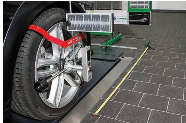
Figure 3.179 This unique, cost effective Camera System Calibration (CSC) tool is quick and simple-to-use and allows precise recalibration of the vehicle's ADAS components. (Source: Hella-Gutmann Solutions)
