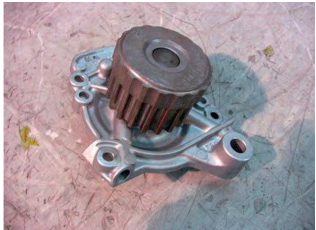
Figure 2.165 Water pump drive gear (cam belt)
