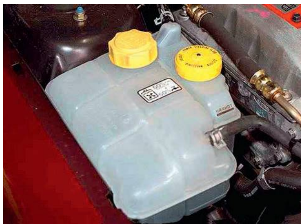
Figure 2.160 Remote expansion tank (on the left)
