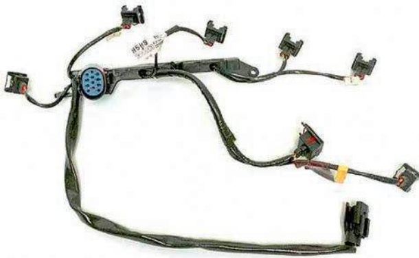
Figure 2.238 Injection wiring harness
