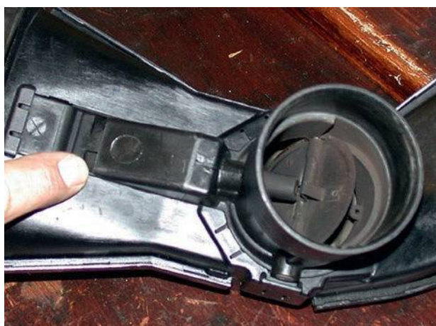
Figure 2.190 Warm-air control (vacuum type)
