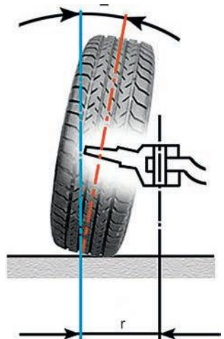
Figure 4.66 Negative camber ( r = scrub radius)
