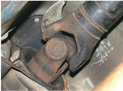
Figure 5.80 Universal joint in position
