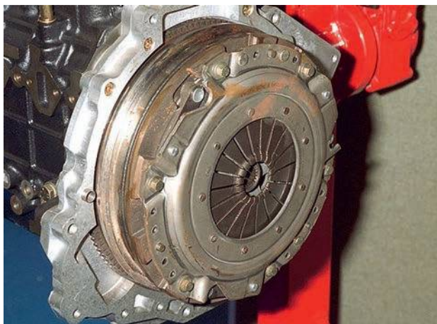
Figure 5.1 The clutch cover is bolted to the engine flywheel
