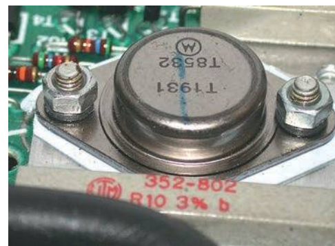
Figure 3.38 Transistor in an electronic control unit
