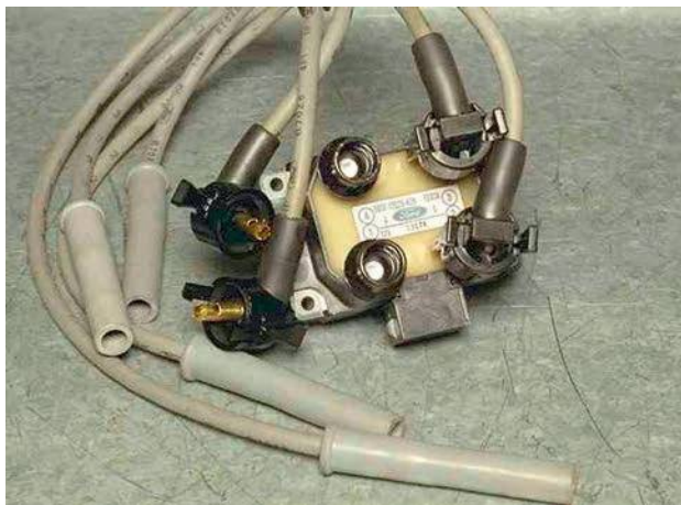
Figure 2.311 Distributorless ignition system (DIS) coil and plug leads
