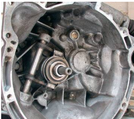
Figure 5.9 Gearbox input shaft around which is the release bearing and its operating lever
