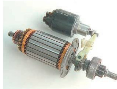
Figure 3.64 One-way clutch behind the drive pinion
