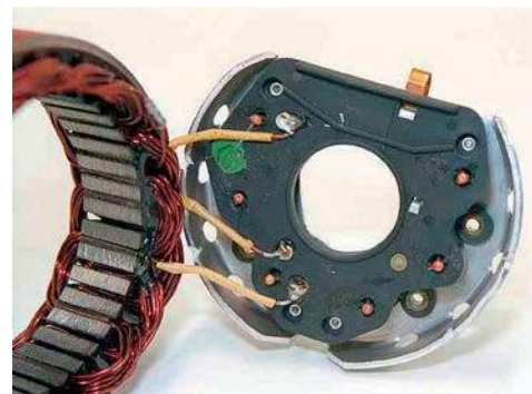
Figure 3.37 Diodes are one-way valves for electricity
