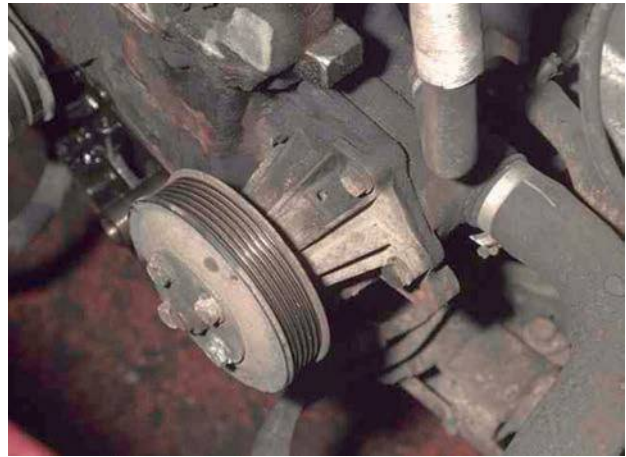
Figure 2.164 External water pump
