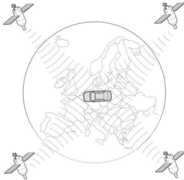
Figure 3.158 Four satellites determine vehicle position more accurately
