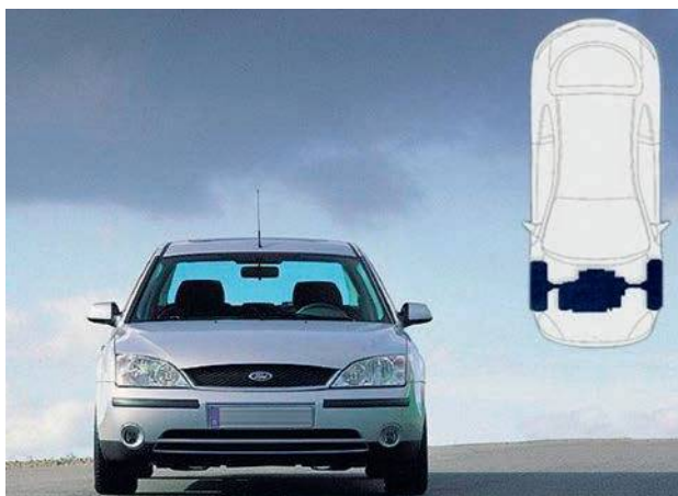
Figure 1.1 Front-engine, front-wheel drive
