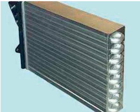
Figure 2.162 The heater matrix (radiator) is similar to the main radiator but smaller
