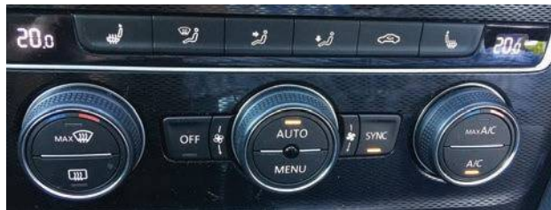
Figure 2.174 Air flow and heater controls
