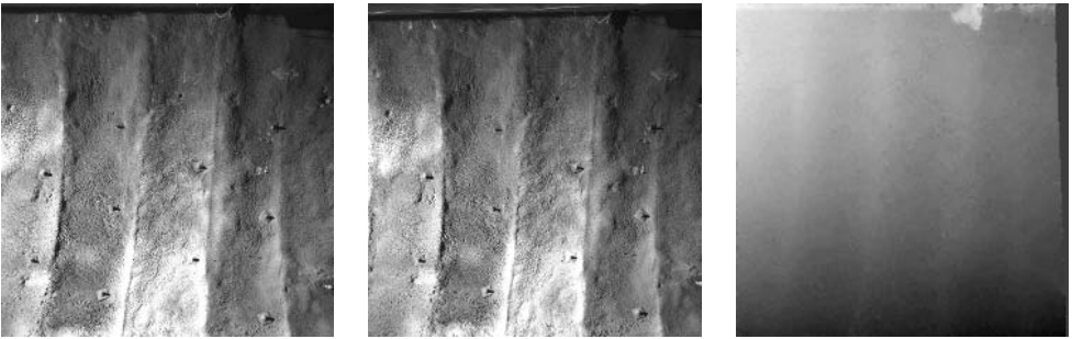
FIGURE 16.9. Image examples: Left and right stereo partner and row disparity image (disparities coded as gray levels) of a concrete surface.
