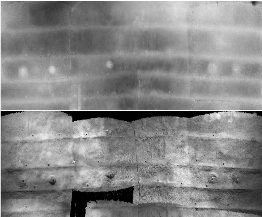
FIGURE 16.10. Result of merging four stereo reconstructions: Ortho image and raster DEM (gray level coded) projected on a cylindrical surface.
