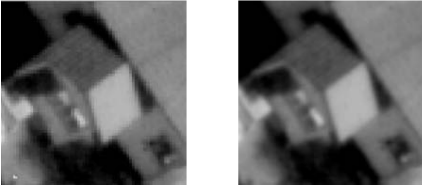
FIGURE 15.2. A small section of an aerial image scanned at 15\ \mu\text{m} and enlarged in a zooming viewer. Left : Nearest neighborhood resampling; right : Bilinear resampling. The right image looks significantly smoother which shows that subpixel information is contained in the image.
