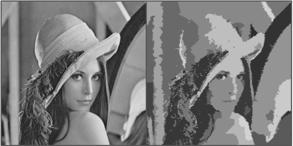
FIGURE 7.5. Image “Lenna”; final result of the segmentation. Starting with 9033 Voronoi polygons 50 regions remain.
