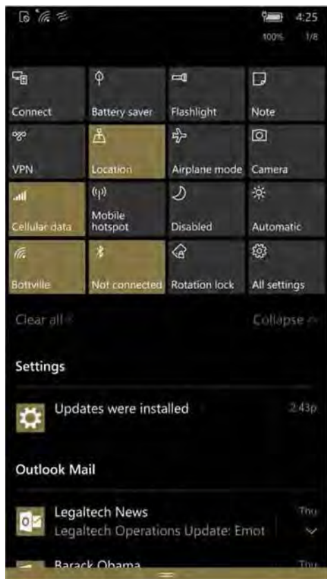
FIGURE 14-5 Just as in Windows 10 on the desktop, the Notifications center contains action buttons for one-tap access to common settings.
