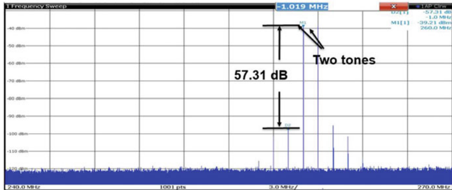
Fig. 6.14 Measured IM_3 at 260 MHz, V_c = 1.1 V, with tones separated by 1 MHz
