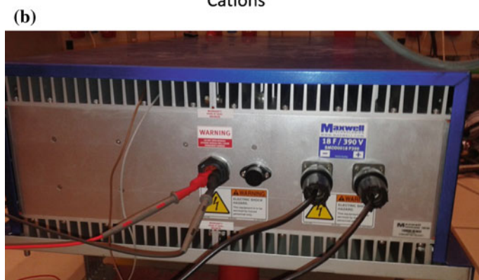
Fig. 10.2 EDLC technology. a Basic cells structure. b 18F/380 V EDLC stack under test at the ESD-Lab sited in the Engineering School of Seville's University
