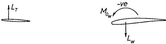
FIG. 3.6. A "tail-first" aeroplane. At zero total lift there must be an up-load on the forward "tail" to produce an overall nose-up moment.
