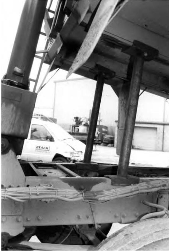
Figure 5.14 Prop (scotch) under raised body of tipper lorry. (Courtesy T E Beach Ltd.)
