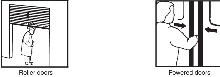
Figure 6.18 Diagrams of the application of pressure sensitive edge strip to prevent injury. (Courtesy EJA Ltd., Nelsa Machine Guarding Systems.)
