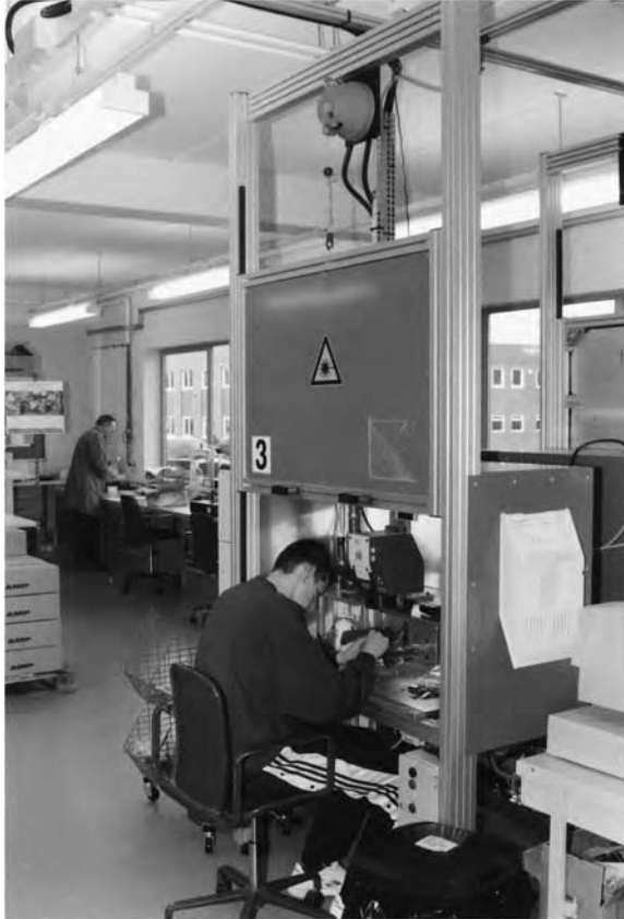
Figure 5.3 Vertical sliding guard supported by a constant tension spring device. (Courtesy of Semi Conductor Tooling Ltd.) Note this guard is fitted to a laser welding booth and is provided with an interlocking proximity switch at its bottom right hand corner that prevents the laser firing until the guard is fully closed.
