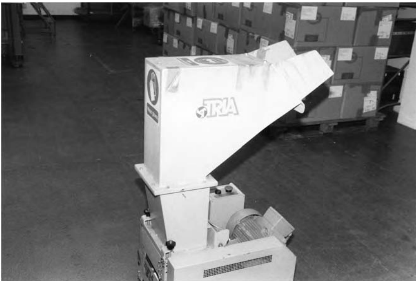
Figure 5.10 A tunnel guard at feed to a plastic granulator extended and cranked to prevent reaching to the cutters. (Courtesy of The Alan Group.)
