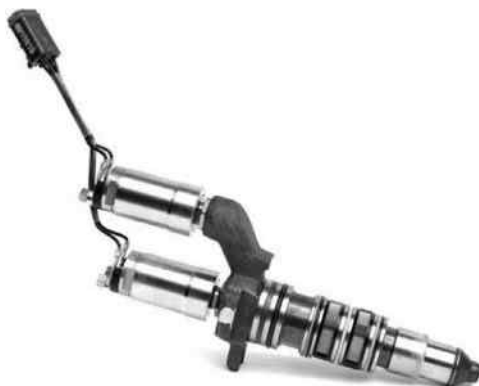
FIGURE 12.12 Westport high-pressure direct injection injector.
