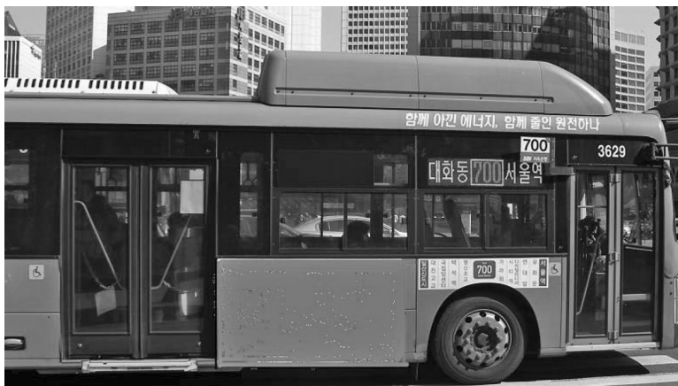
FIGURE 5.2 An example of a city bus powered with a dual-fuel engine by having the cylinders of compressed natural gas installed on its roof.
