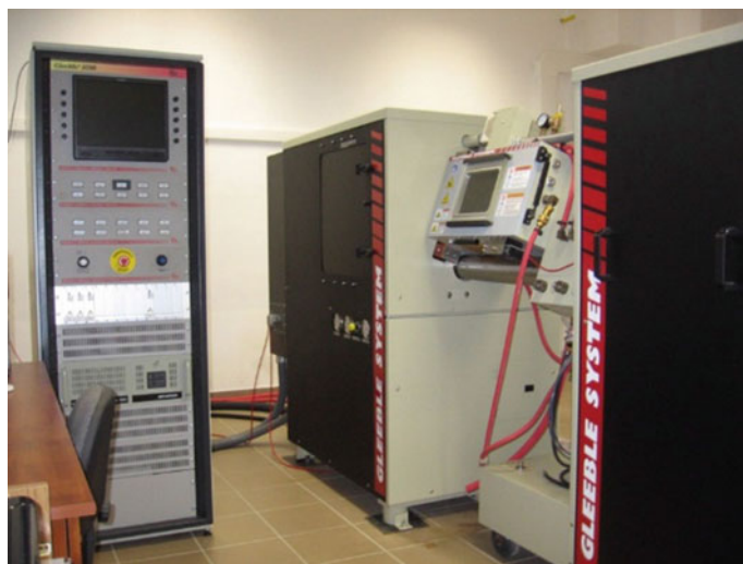
Fig. 2 Gleeble 3500 thermo-mechanical, physical simulator installed at the University of Miskolc
