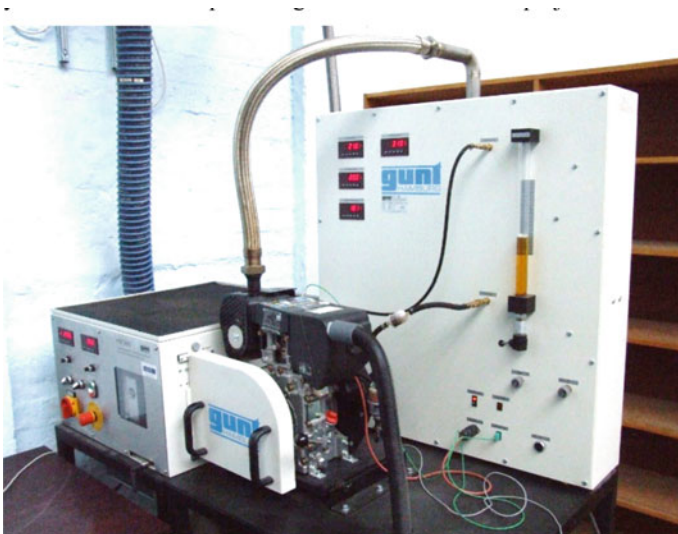
Fig. 8 An engine test lab system with a drive motor and dynamometer produced by GUNT (2010)
