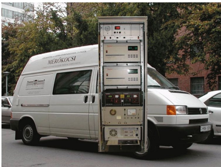
Fig. 2 The portable emission measuring laboratory
