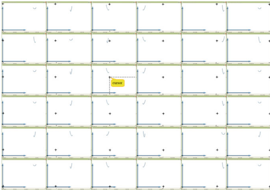
Fig. 6 Checking against undercut using Fi2 functions
