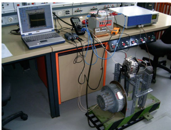
Fig. 14 Laboratory measurement of the alternator
