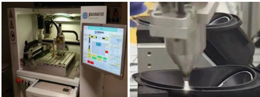
Fig. 7 The open air atmospheric plasma jet laboratory apparatus (Plasmatreater AS 400) installed in the Surface Techniques Laboratory (Institute of Metallurgy)/left/. An industrial application example of using plasma jet for surface fine cleaning and surface modification/activation before gluing and sealing a car headlight housing/right/[8]
