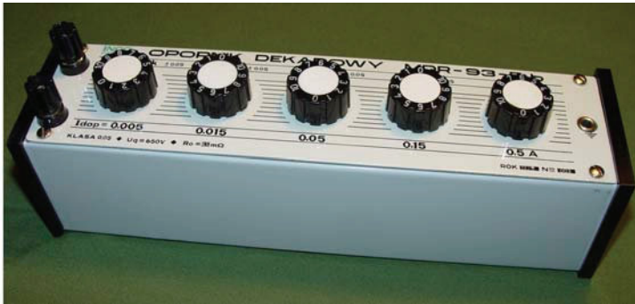
Figure 2.39. An example of the resistor decade box
