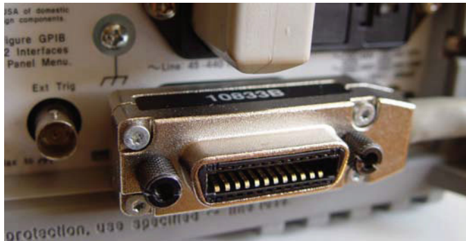
Figure 6.34. The connector of GPIB interface
