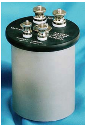
Figure 2.37. An example of the standard resistor – model 5615 of Tinsley (Tinsley 2005) (permission of Tinsley Precise Instruments)
