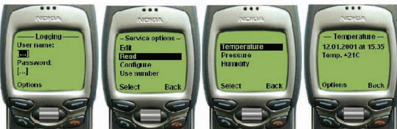
Figure 6.48. The measuring system using GSM communication and WAP technology (Winiecki 2003)
