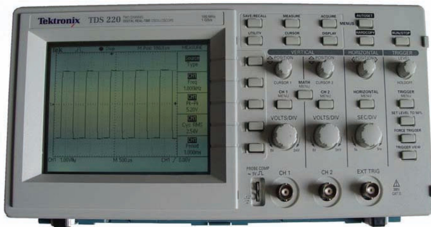
Figure 5.144. The example of the digital oscilloscope – oscilloscope of Tektronix (Tektronix 2005)
