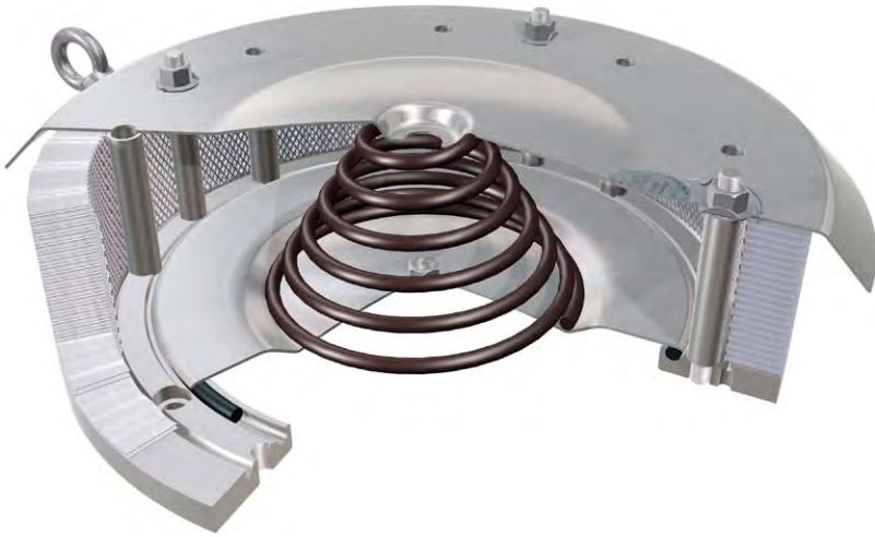
FIGURE 32.3 The large relief cross-section of a Hoerbiger valve allows explosion waves to disperse freely and rapidly; the low mass, frictionless guided valve plate opens in fractions of a second and then closes tightly to prevent the inrush of air (oxygen); and an integrated flame absorber prevents the escape of blast flames
