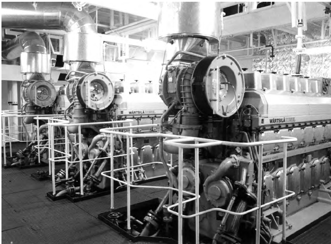
FIGURE 27.10 Three Wärtsilä 6L20-powered gensets in the engine room of a feeder container ship
