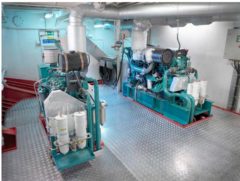
FIGURE 30.45 Two Volvo Penta D16 MH engines arranged to power a double-ended road ferry
