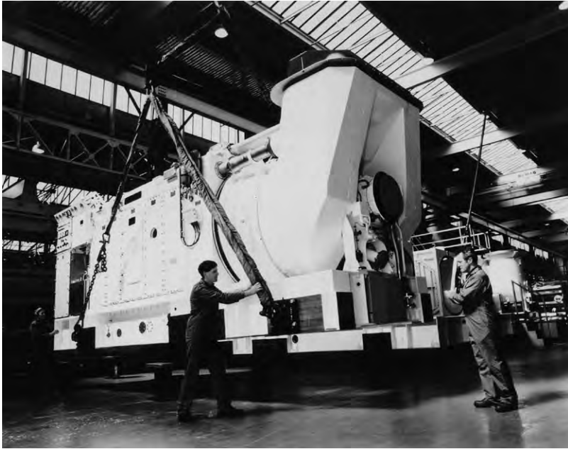
FIGURE 31.17 A fully packaged Rolls-Royce Marine Spey propulsion module
