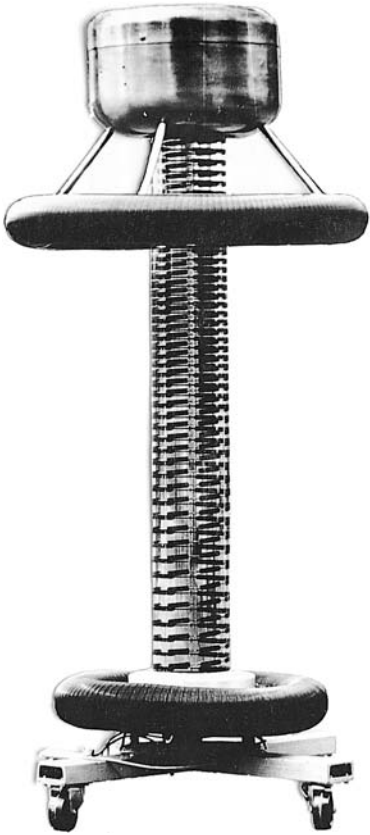
Figure 3.10 300-kV divider for d.c. height 210 cm (PTB, Germany) (35)
