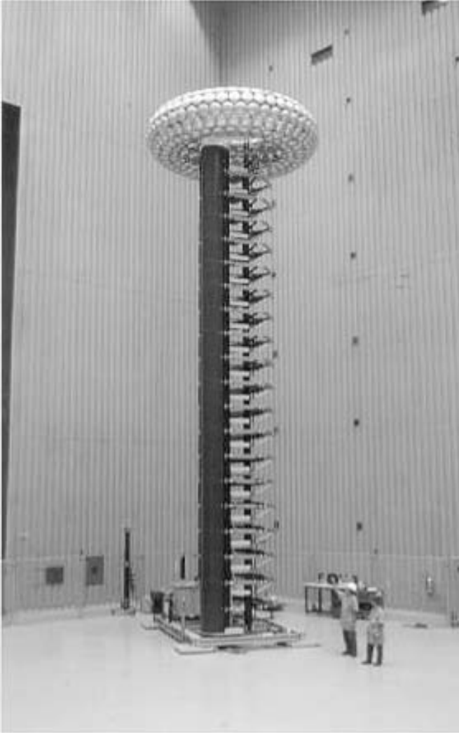
Figure 2.34 Indoor impulse generator, 20-stage, 4-MV, 200-kJ, with encapsulated sphere gaps (courtesy of CEPEL, Rio de Janeiro, manufactured by Haefely)
