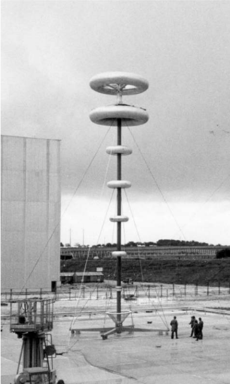
Figure 3.41 Series-damped capacitor voltage divider for 6-MV impulse voltage (courtesy EdF, Les Renardieres, France)
