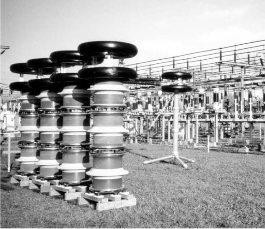
Figure 2.22 Modular reactors of a series resonant circuit with variable frequency during an on-site test of very long polymeric cables (courtesy FKH, Zurich, Switzerland)
