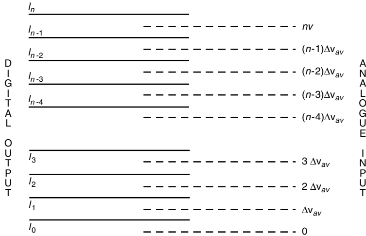
Figure 3.49 Analogue input to digital output relation of an ideal A/D converter
