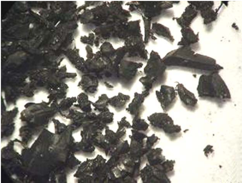
9.1 Rubber particles as observed with a stereoscope (magnification \times 40 ).
