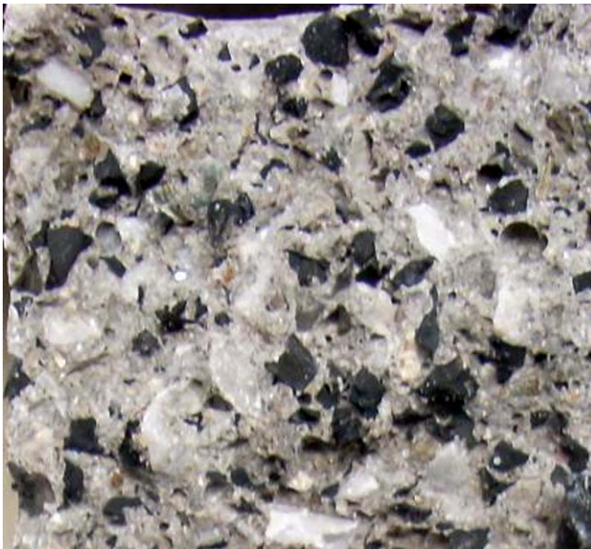
9.3 Rubber distribution in rubberised concrete mixture.
