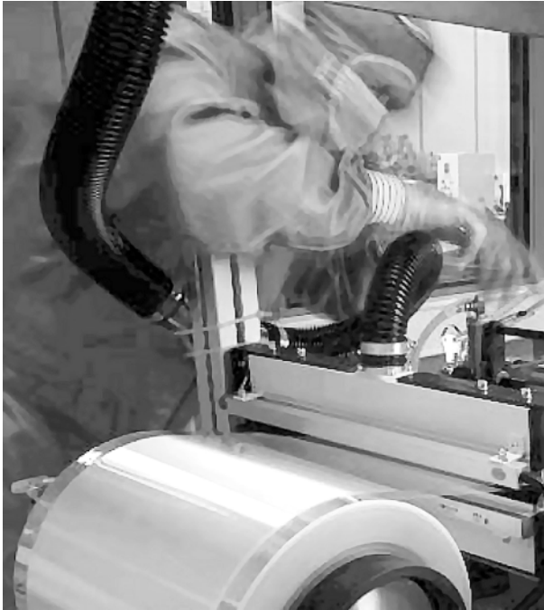
11.3 Industrial production of DEAP sensor. Courtesy of Danfoss PolyPower A/S, Denmark.
