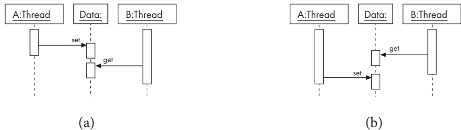
Figure 10.6 A critical race situation caused by a change in speed of execution
