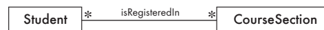
Figure 5.6 A many-to-many association. The ‘grade’ attribute can be put in neither class
