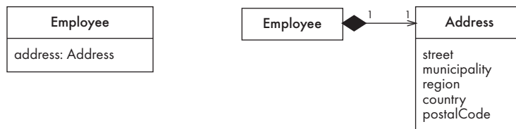
Figure 5.20 The address of an employee represented as an attribute or as a composition
