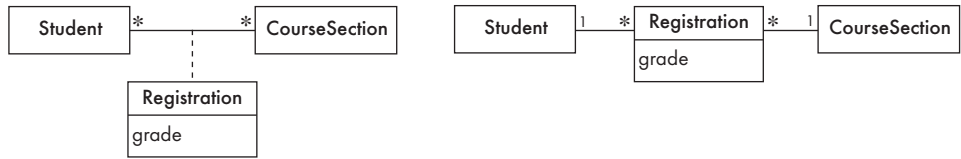
Figure 5.7 A many-to-many association with an association class, and an equivalent diagram using two one-to-many associations
