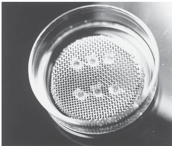
Fig. 2. The Trowell-type organ culture dish. The metal grid supports six pieces of filters. The cultured explants (like the one in the bottom of Fig. 1 ) are seen on the filters over the holes of the grid.
