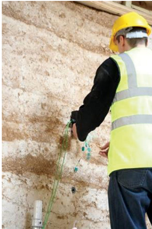
Figure 3.8 Thermocouples being placed into the rammed earth wall at Hill Holt Wood Centre, near Lincoln, UK (Photo by Steve Goodhew).
