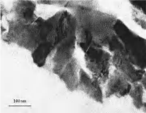
Figure 4: A bright field HRTEM of grains in film at Mo/CIGS interface. Mo delaminated during sample preparation leaving only the CIGS film.
