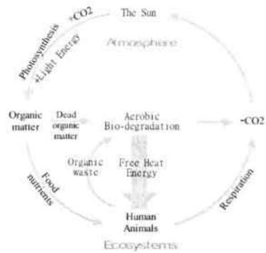
Figure 3. Reclaiming the free heat energy from aerobic bio-degradation.
