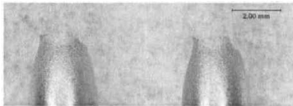
Figure IV. Optical photograph of gage section of X60 line pipe steel specimen tested in SFGE containing an SCC inhibitor (500 ppm of 30% NH 4 OH).
