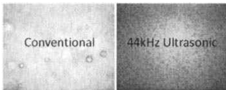
Figure 4. Visual comparison between conventional shear mixing and ultrasonic mixing at 44 kHz.
